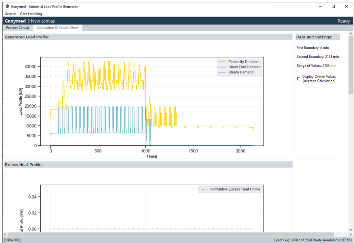
Figure 21: Generated synthetic LPs in the calculations and results sheet.
