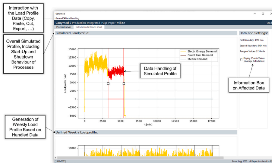
Fig. 16. Ganymed GUI Calculation & Results Sheet.
