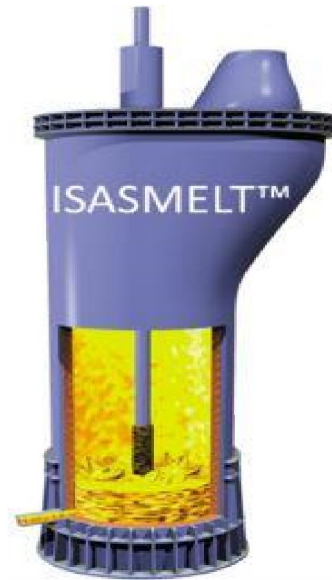
Figure 2.2 Cross sectional view of the isasmelt furnace via xstrata technology. [19]
