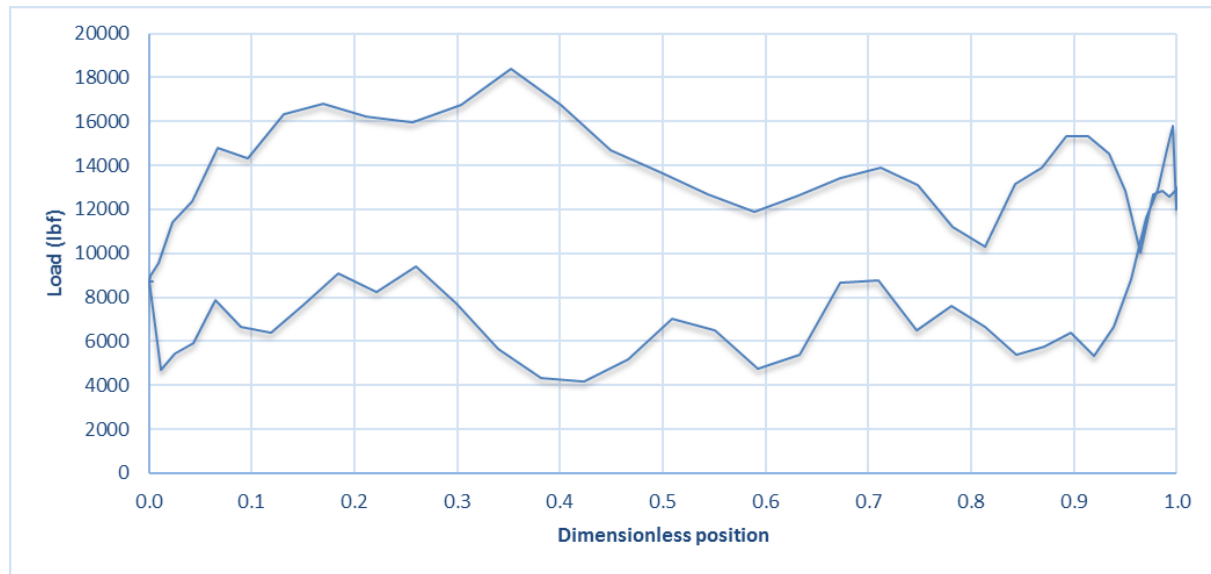
Figure 22: Dynamometer Card – Conventional Unit / CSR
