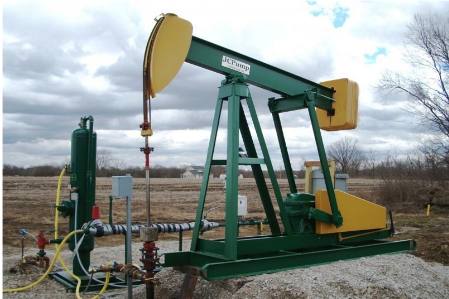
Figure 7. Example of Beam-balanced Pumping Unit [10]
