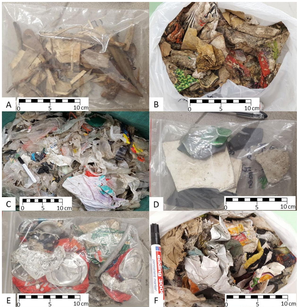
Figure A3. Exemplary photos of the manually sorted material fractions: wood—A; P&C—B; plastics—C; inert—D; metals—E; others—F.
