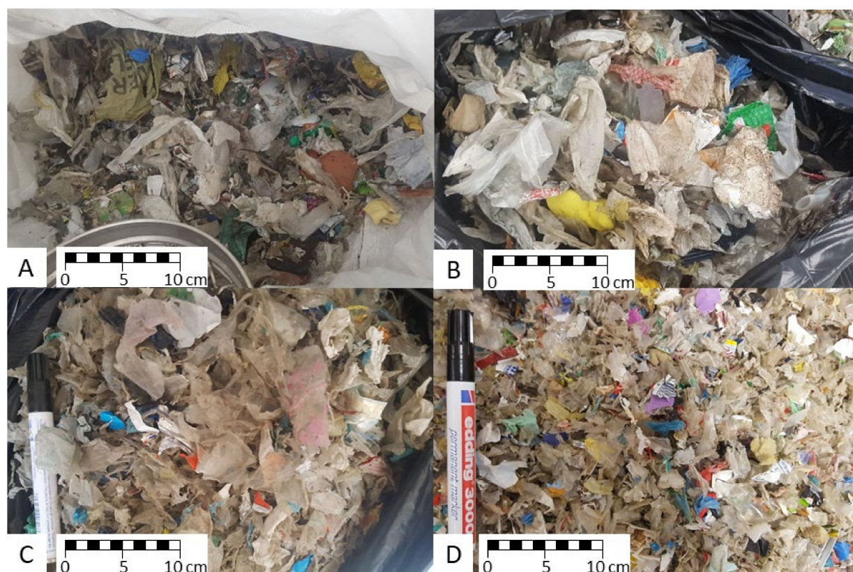
Figure A2. Exemplary photos of the input materials: SRF in (A) and (B), PO_A in (C), and PO_B in (D).
