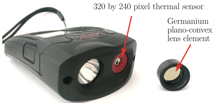
Figure 3.10: A macro lens was fitted to a thermal imaging camera to allow the measurement of the cross section temperature of rubber strands 3.5 mm in diameter.
