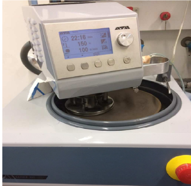
Figure 69: The ATM Saphir 520 polishing machine.
