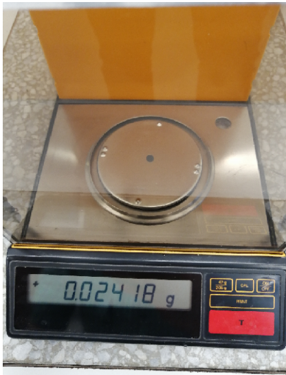
(a) Weighting the prepared samples for DSC tests
