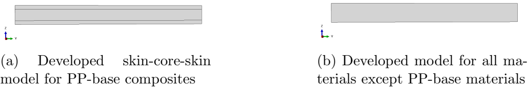
Figure 3.3.3: The developed models considering the fibre distribution in the direction of thickness
