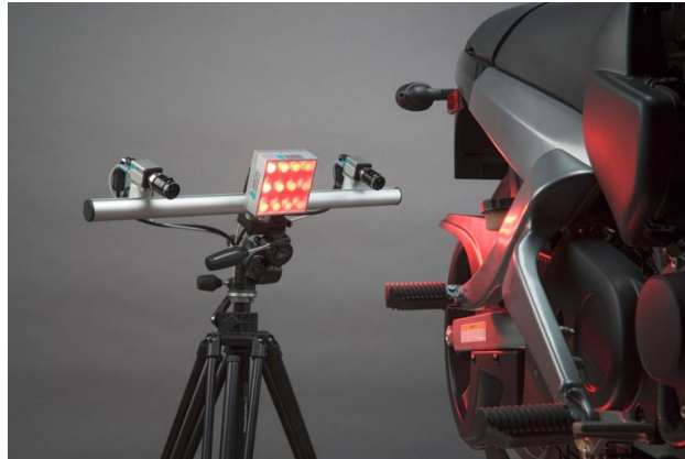
(a) Used DanTec - Solid Mechanics DIC device for measuring thermal expansions [61]
