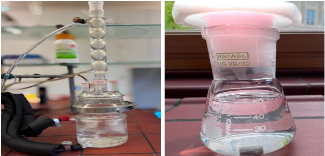
Figure 3.11: Testing cell and flask with specimen for immersion test
