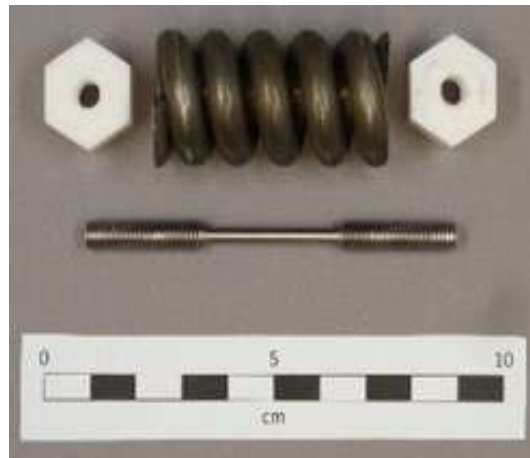
Figure 3.12: Small tensile specimen with spring and nuts for constant load test (CLT)
