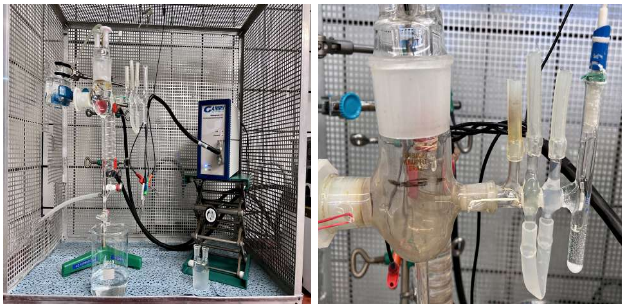
Figure 3.10: Experimental setup and corrosion cell used to perform potentiodynamic tests
