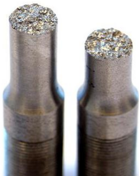
Figure 2. 73: Brittle fracture appearance [242].
