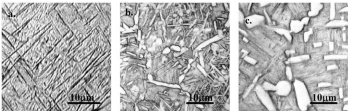
Figure 2. 43: Effect of water quenching on microstructure of Ti6Al4V heat treated at different temperature (a) 1100°C, (b) 950°C, (c) 900°C [161], [162].
