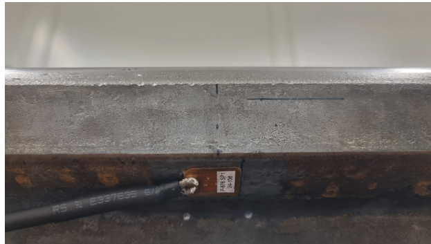
Fig. 6.4: Piezoelectric transducer glued to the bottom side of a laboratory specimen's rail head.
