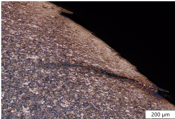
(a) Micrograph of the rail specimen subjected to N = 50000 load cycles, showing the identified head check, captured at 100x magnification. This specimen exhibited only a single head check with a depth a = 394\ \mu\text{m} .
