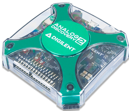
(a) Image of the USB oscilloscope, Analog Discovery 2 , which forms the core of the measurement device [54].
