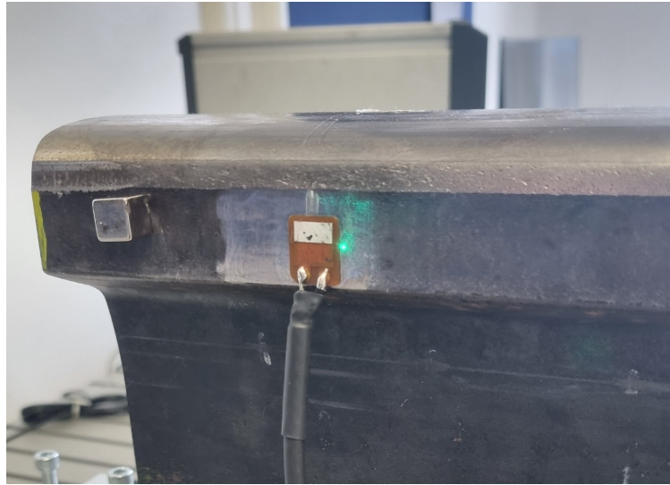
Fig. 6.12: Experimental setup to characterize the velocity v and the attenuation behavior of SAWs propagating on the rail head: The piezoelectric transducer was affixed to the inside of the rail head. A green laser indicates the LDV's sensing position at the time the photograph was captured. The illustrated setup represents a distance d from the edge of the piezoelectric transducer d = 0 mm. Measurements were performed within the distance range from d_{min} = 20 mm to d_{max} = 300 mm with increments of \Delta d = 20 mm.
