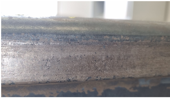
(a) The rail head's surface on the inside of the rail was mostly close to the initial as-rolled state.
