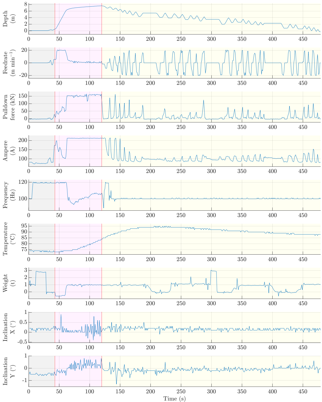
Fig. 5.2: Example time-series plot of all 9 channels of the vibro ground improvement process. The process is segmented into an initial phase (grey), a penetration phase (pink) and a compaction phase (yellow).
