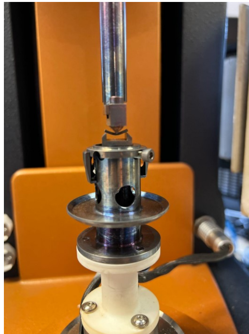
Figure 9: 3-point bending DMA experiment test setup showing the deflection of a specimen after the completion of the experiment.
