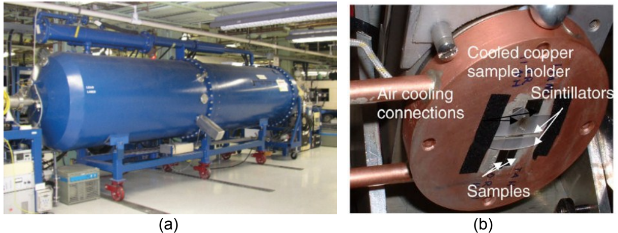
Figure 8. (a) Tandem ion accelerator at IBML in LANL [36]. (b) Sample mounting in the ion beam irradiation experiment [38].
