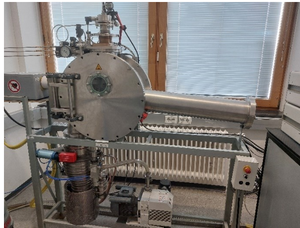
Figure 3-2: Melt spinning machine at the Chair of Casting Research.
