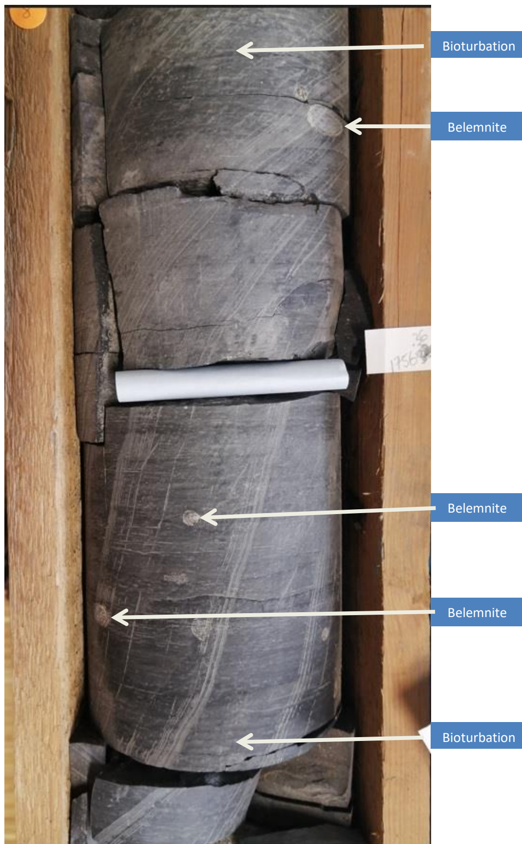
Fig. A8. Drill core section showing increased amounts of belemnite fossils and bioturbation structures in the uppermost Falciferum sub-zone.
