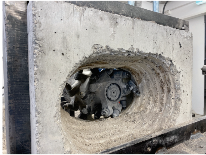
Figure 4.14: Partly cut test specimen
