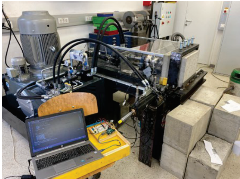
Figure 4.4: Cutter head test rig assembly with measurement system and rock samples
