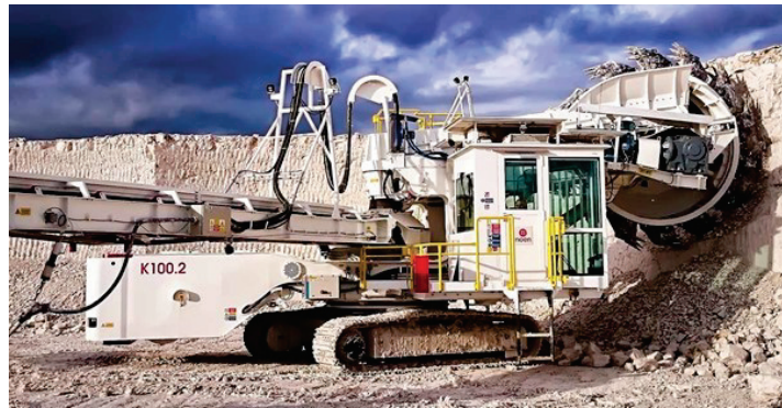
Figure A.29: Compact bucket wheel excavator © Noen [190]
