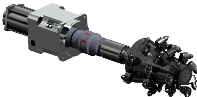
Figure 7.7: Part-face cutting tool - Concept
