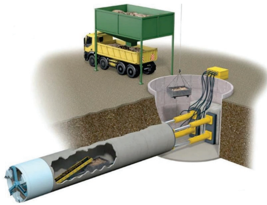
Figure A.19: Pipe jacking arrangement © PipeJackingAssociation [182]
