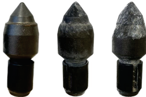
Figure 4.32: New pick (left), pick with minor wear (center) and pick with major wear (right)
