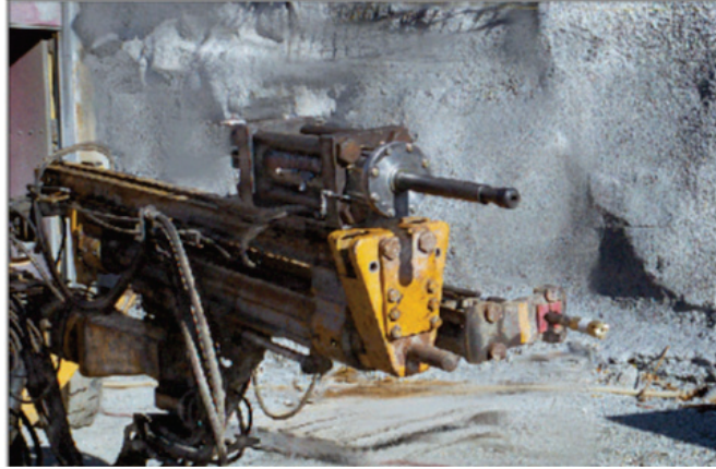
Figure 2.7: Controlled foam injection barrel and drill steel [34]
