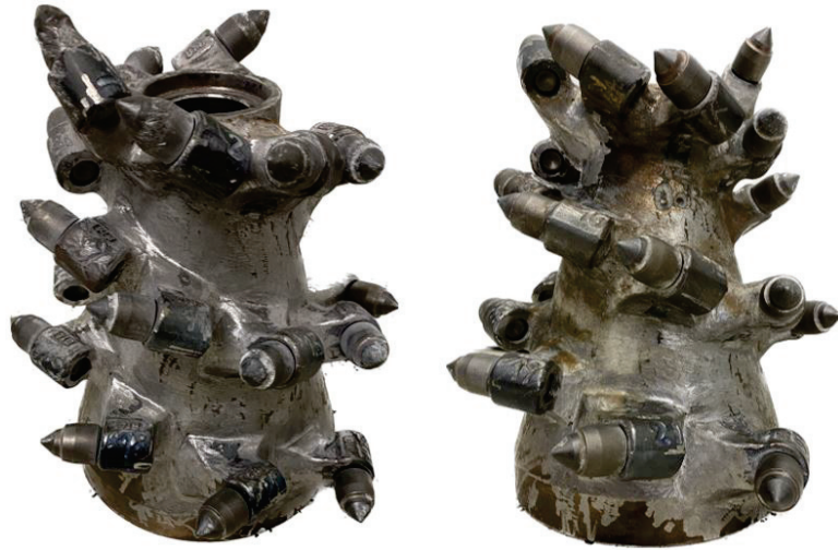
Figure 4.18: Original (left) and adapted (right) cutter head
