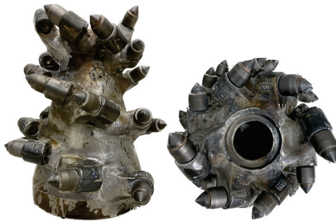
Figure 4.7: Adapted cutter head with 24 picks
