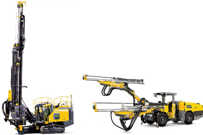
Figure A.5: Surface drilling rig (left) and underground drill jumbo (right) © Epiroc [85]
