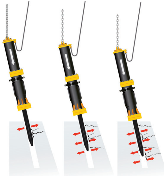
Figure A.22: Hydraulic rock splitter © Yamamoto [184]
