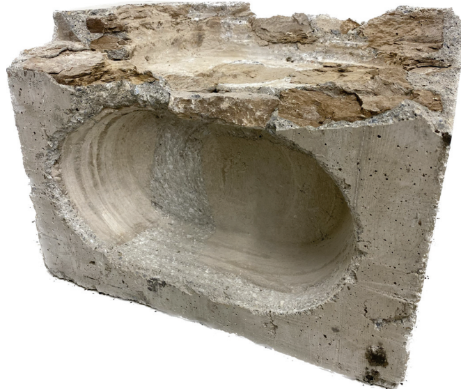
Figure 4.12: Test specimen with oilshale layers and limestone insertions
