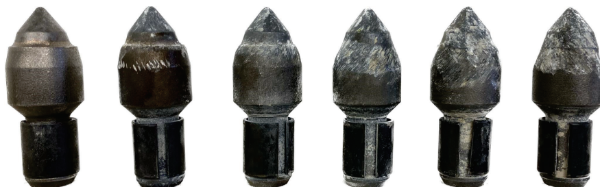
Figure 4.33: Increasing wear on conical pick tools
