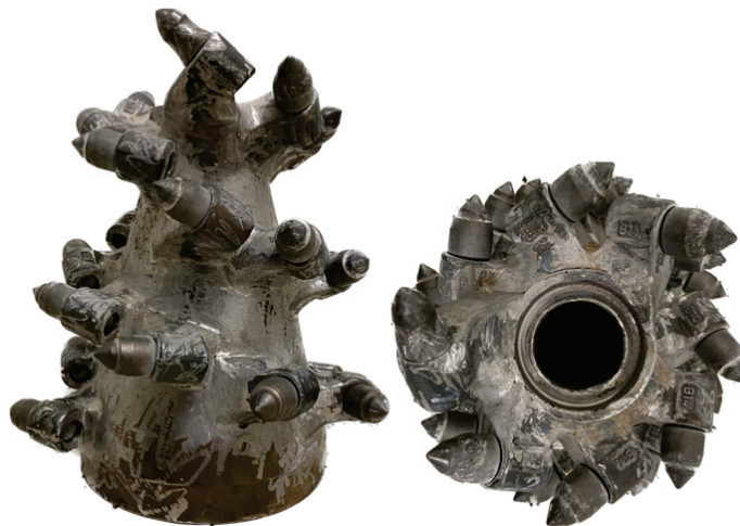
Figure 4.6: Original cutter head with 23 picks
