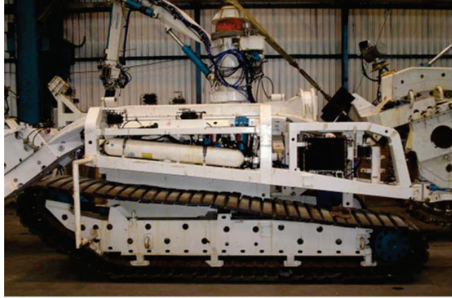
Figure 2.13: Tracked subsea trencher (T3) [71]
