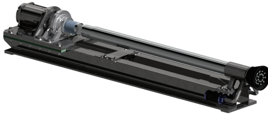
Figure 7.3: Water-hydraulic rotary-percussive rock drill - Concept
