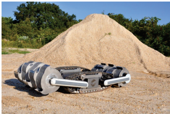
Figure 2.10: NASA Rassor field test [66]
