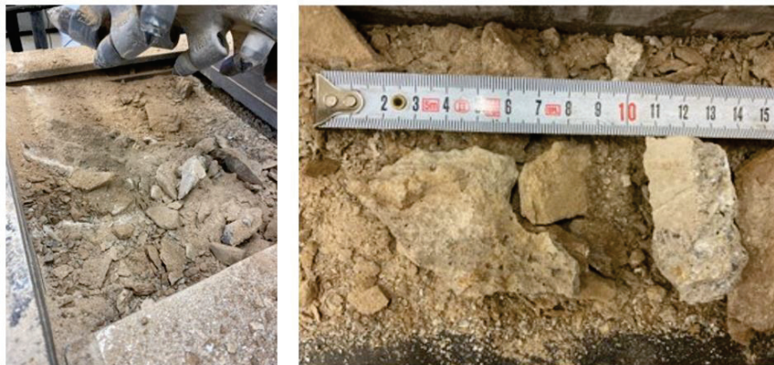
Figure 4.31: Debris of oilshale sample
