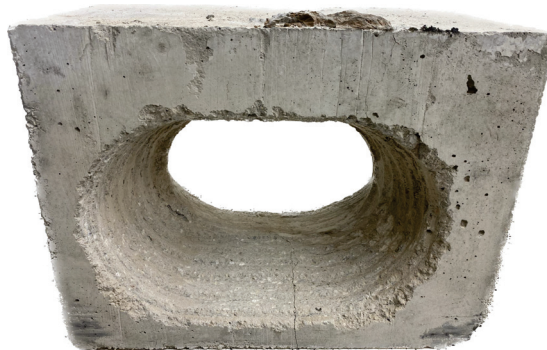
Figure 4.11: Cut specimen with oilshale insertions
