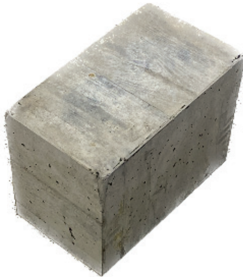
Figure 4.9: Test specimen - 400 x 230 x 300 mm (w x l x h)
