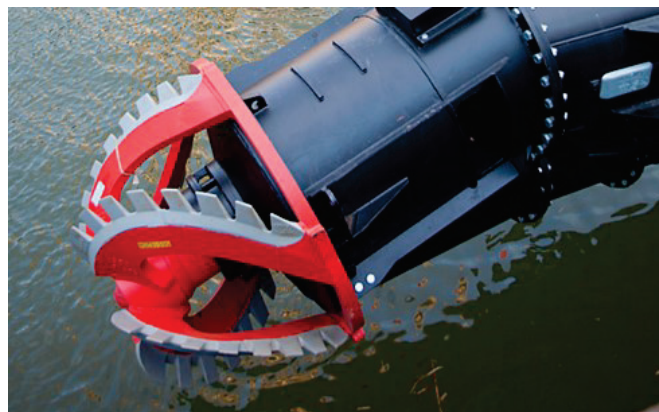
Figure A.28: Cutter head of a hydraulic suction dredger © RoyalIHC [188]
