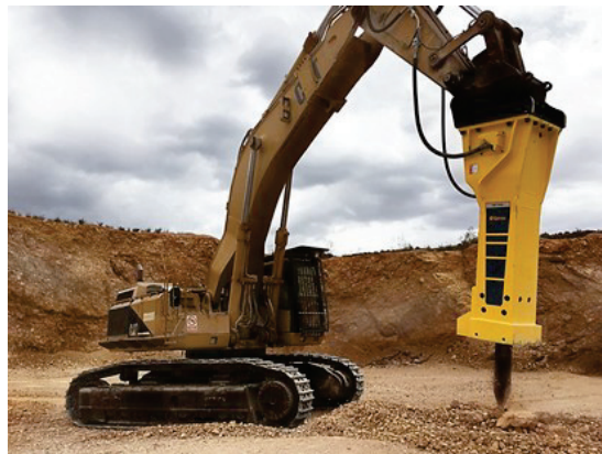
Figure A.23: Hydraulic rock breaker mounted on excavator © Epiroc [85]
