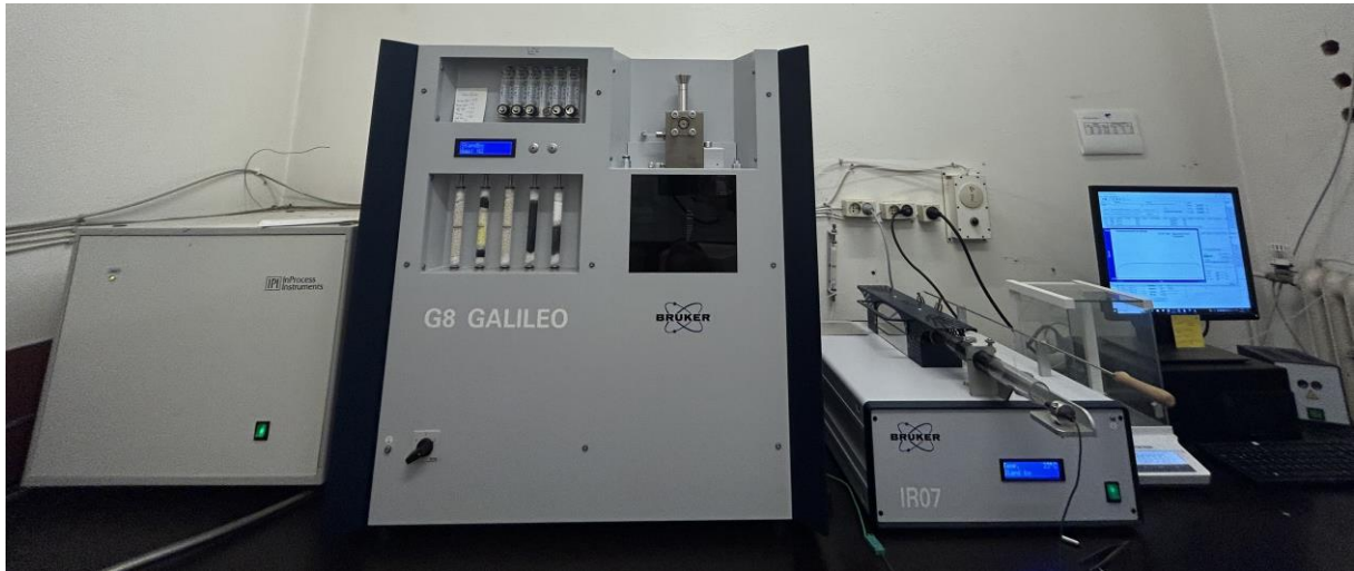
Figure 45: TDS with mass spectrometer
