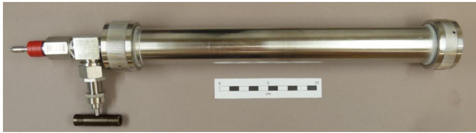
Figure 34: Autoclave made of Alloy 625
