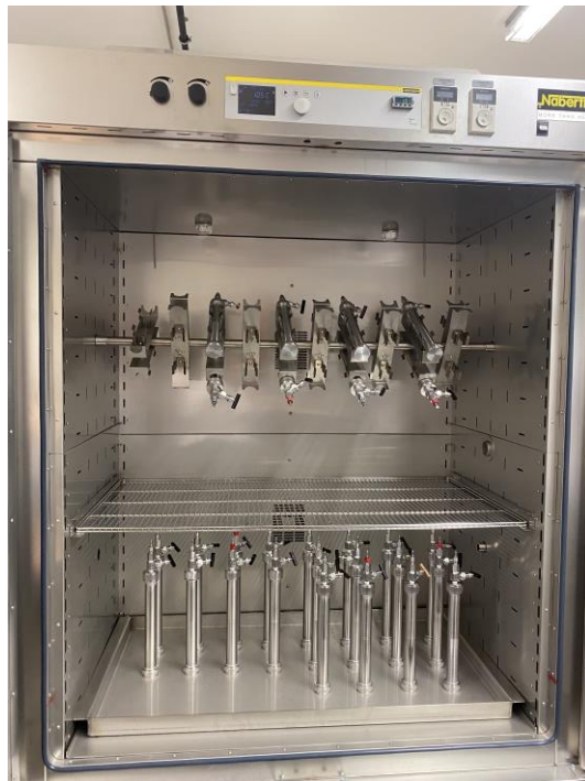
Figure 43: Oven with a rotating shaft and a holder for the autoclave
