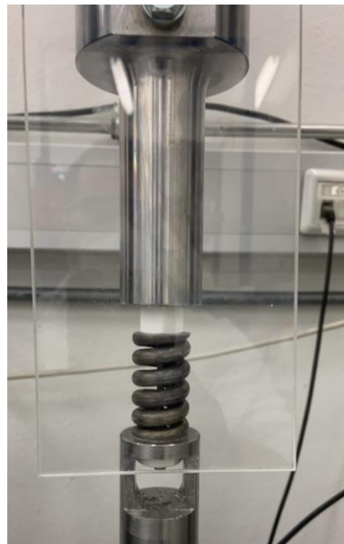
Figure 38: Loading of the tensed specimen with the aid of the clamping device
