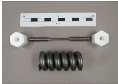
Figure 37: Ceramic nuts, spring and tensile specimen
