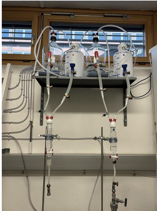
Figure 41: Filling station for dosing the electrolyte
