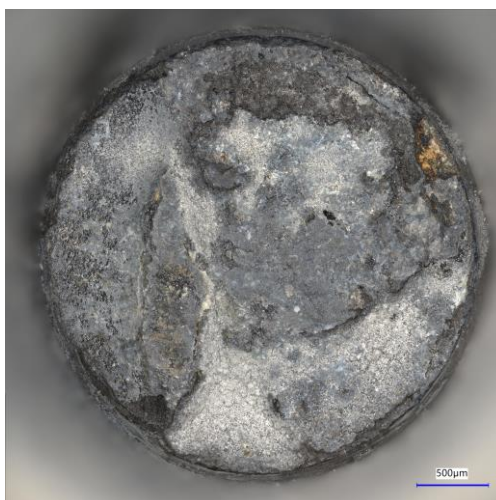
Figure 50: Fracture surface of a quenched material at 120 °C with 200 g/l NaCl in gas D (120 bar H 2 + 15 bar CO 2 + 1 bar H 2 S) and rotating
