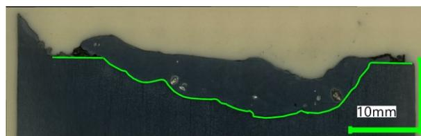
**Figure 102:** Digital microscope image of the 0%-C-DRI-Test (Test 1 - pretest) cross-section
