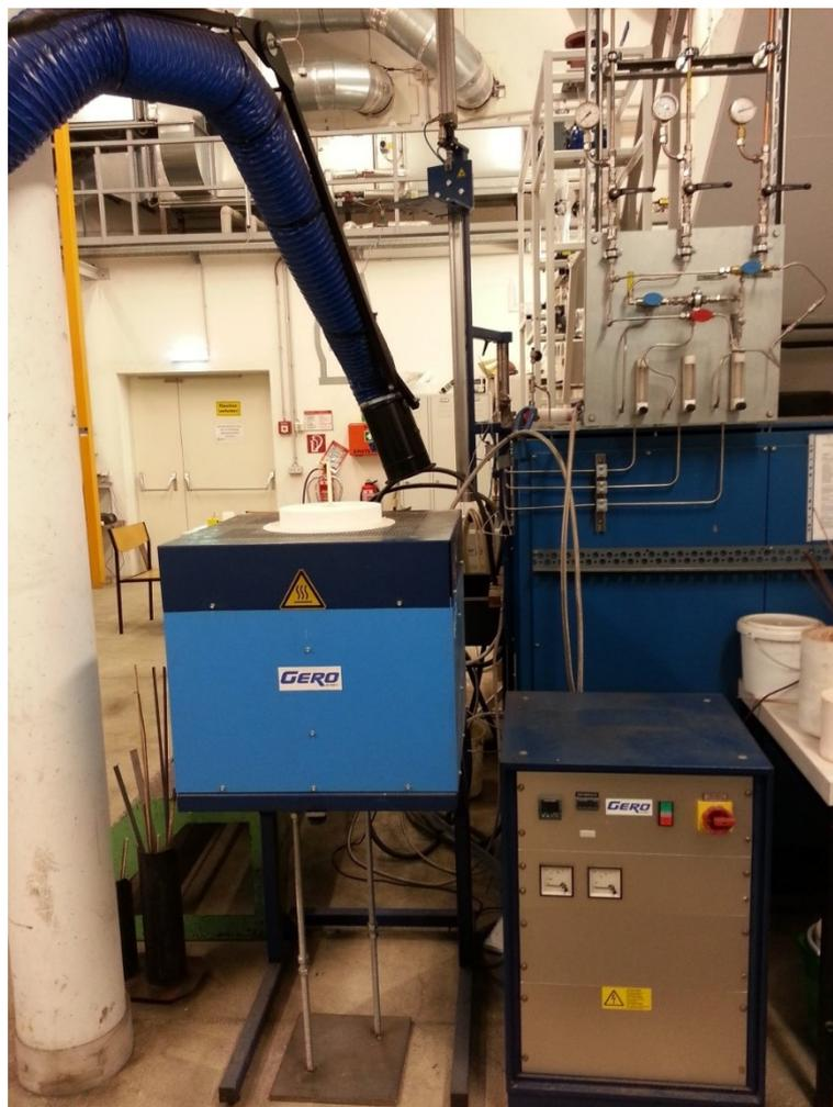
**Figure 25:** Gero® vertical tube furnace
