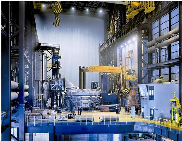
**Figure 6:** Colakoglu melt shop with a Primetals Ultimate EAF ©Primetals<sup>[70]</sup>
