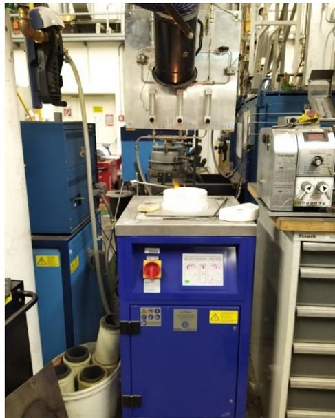
**Figure 20:** MU900 induction furnace
