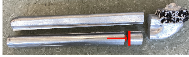
Figure 3.3: As-cast sample for microstructure evaluation sectioned from Diez mould.
