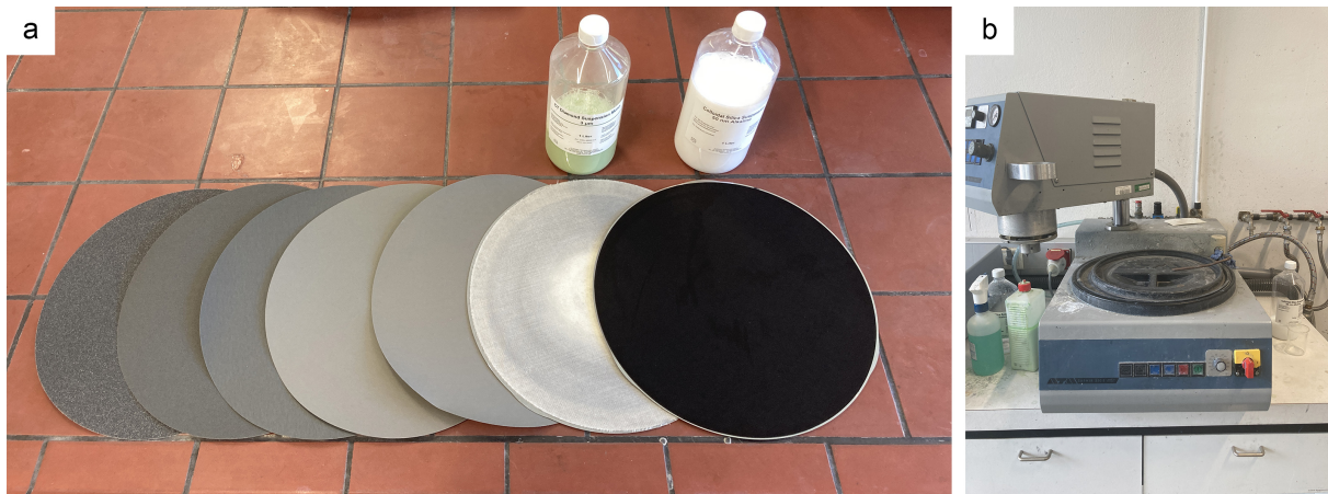
Figure 3.6: (a) Grinding and polishing equipment and (b) grinding and polishing machine at the Chair of Casting Research, Leoben.
