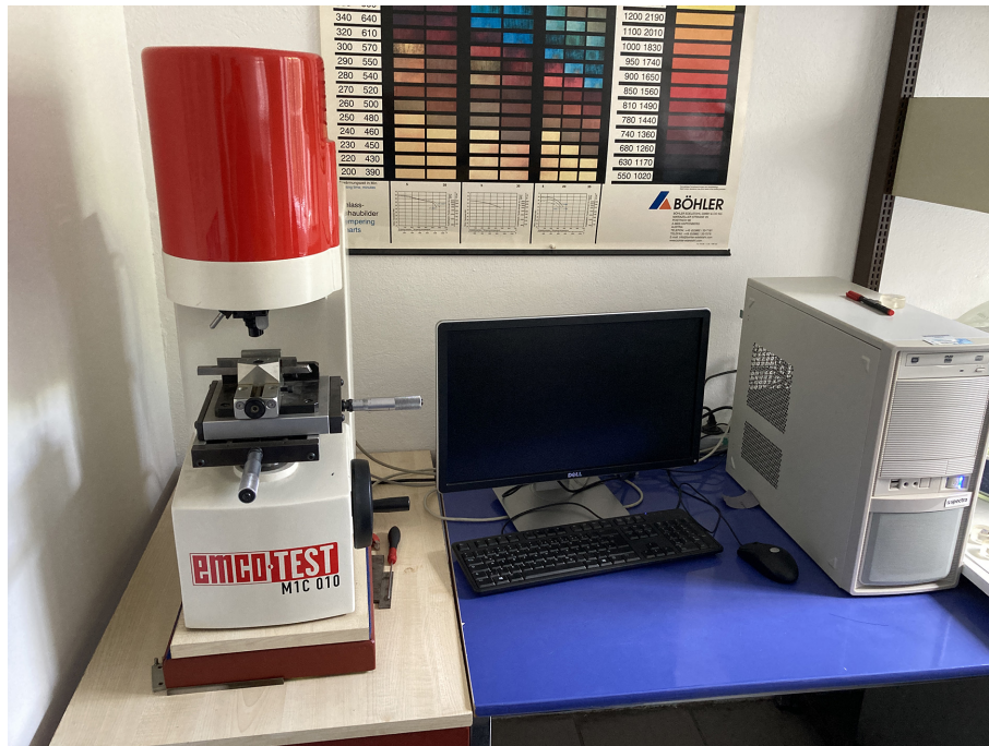
Figure 3.13: Vickers hardness testing machine at the Chair of Metal Forming, Leoben.
