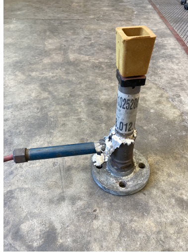
Figure 3.4: Rectangular Croning sand cup including K-type thermocouple on the stand at the Chair of Casting Research, Leoben.
