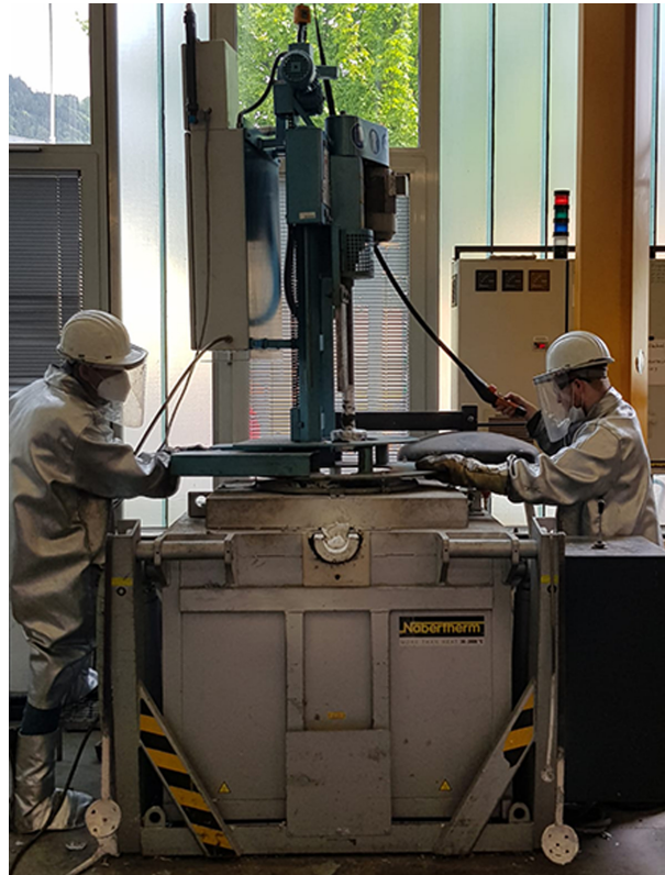
Figure 3.1: FDU (Foundry Degassing Unit) degassing using impeller at the Chair of Casting Research, Leoben.
