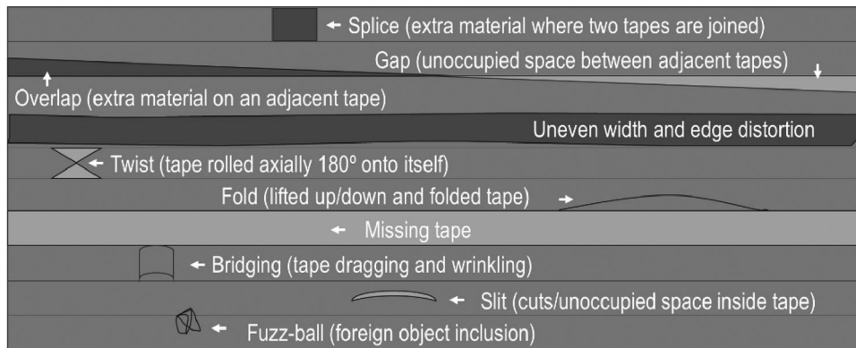
Figure 1. Summary of defects capable of being detected inline via surface or edge detection.
