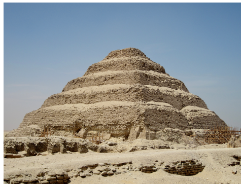
Figure 2.7: Pyramid of Djoser, demonstrating the aliasing effect in building direction due to the discrete layer thickness and limited spatial resolution [46].
