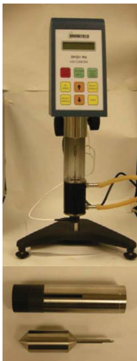
Figure 21: Brookfield viscometer with example beaker and spindle for measurements
