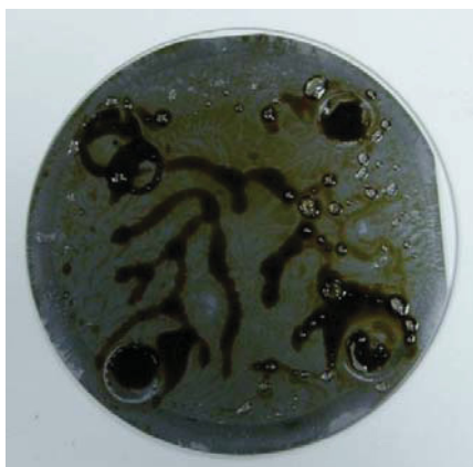
Figure 44: Micromodel reverse side after oil saturation with a leaking O-ring
