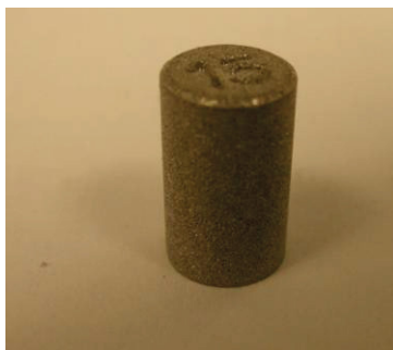
Figure 68: Cartridge filter with 15 microns average filter size
