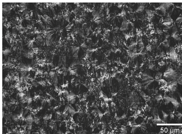
Fig. 63: Illustration of microstructure in the core of a dumbbell tensile multipurpose specimen of RPP(3.5), by polarized light microscopy.
