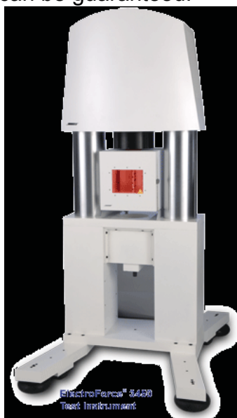
Fig. 28: The Bose Electro Force 3450 DMA testing machine with tempering chamber. (image copied from www.bose-electroforce.com )
