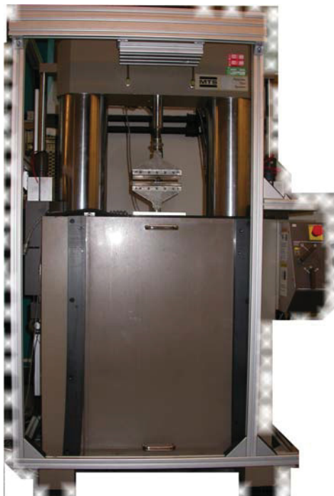
Fig. 25: The servo hydraulic MTS 831.59 Polymer Test System of the Institute of Material Science and Testing of Plastics at the University of Leoben.
