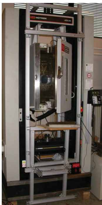
Fig. 23: Instron testing machine, type INSTRON 5500R, (Fa. INSTRON LIMITED; High Wycombe, UK).
