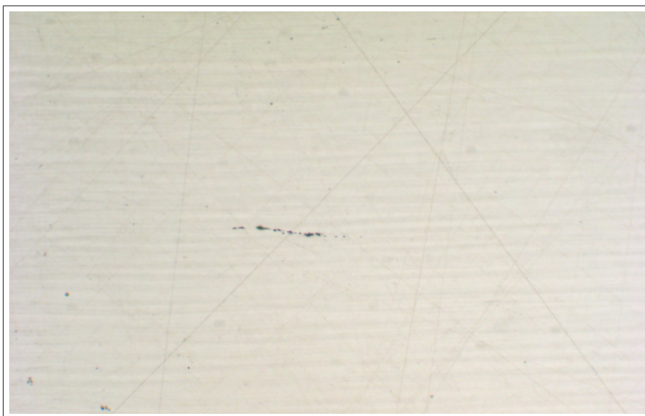
Figure 4.1: Image1: Specimen with inclusion type OA.
