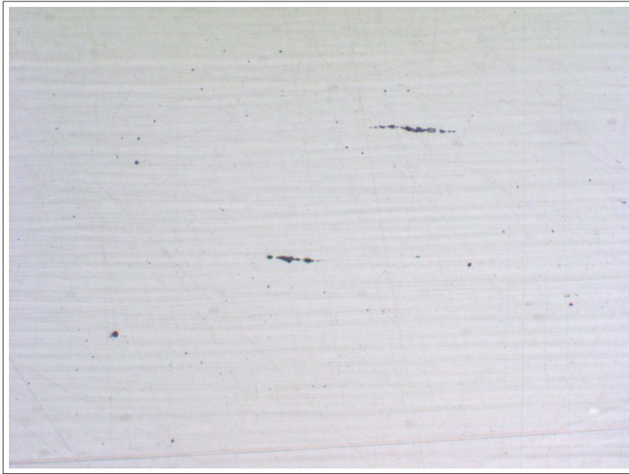
Figure 4.8: Image 4: Specimen with inclusion types OA and OG.
