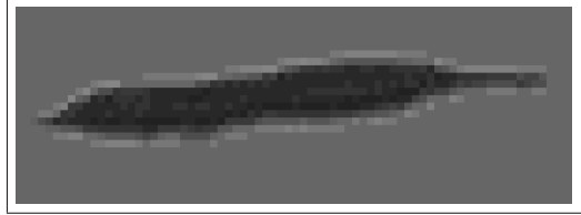
Figure 3.8: Test oxide inclusion to receive adequate threshold values.
