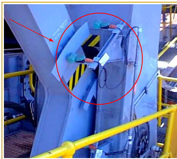
Figure 7-26: Luff- upper / lower limit proximity switch.
