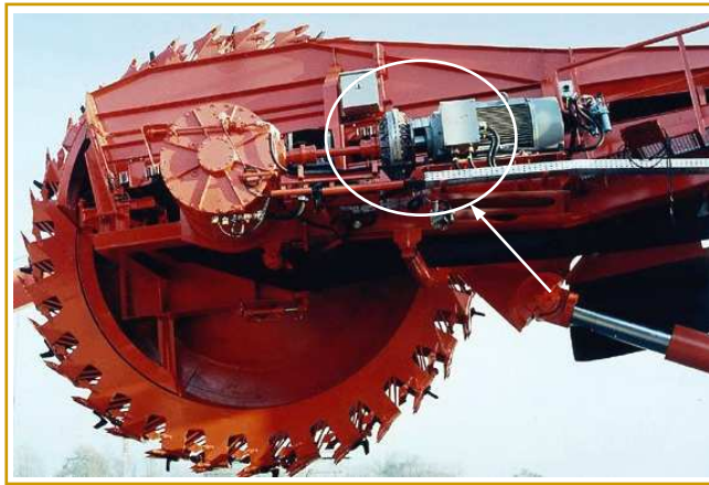
Figure 7-35: Hydraulic coupling between the motor and the gearbox.
