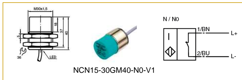
Figure 8-3: Inductive proximity switch with circuit connection.
