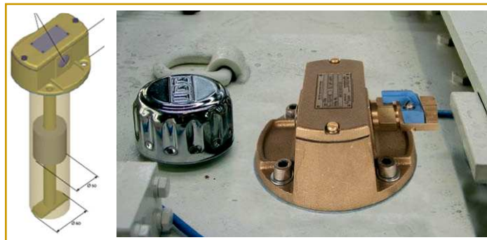
Figure 5-10: Oil level switch (L) and its position at the top of the hydraulic tank (R).
