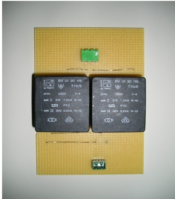
Figure 4.6 Transformer group for 100V voltage
