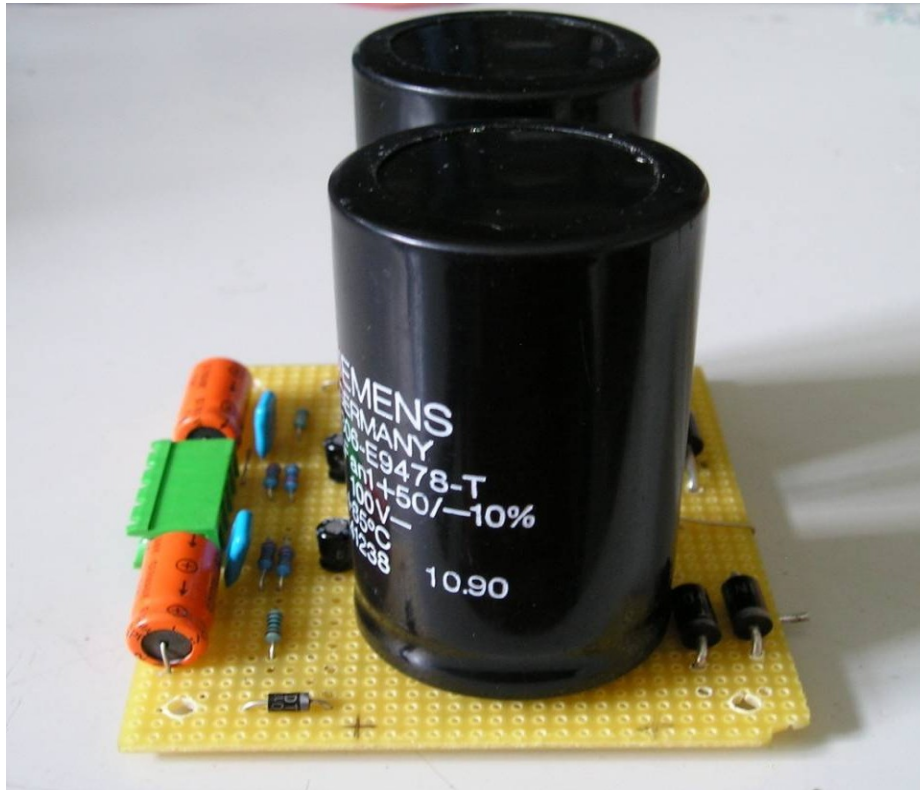
Figure 4.41 Power supply for transducers and amplifiers
