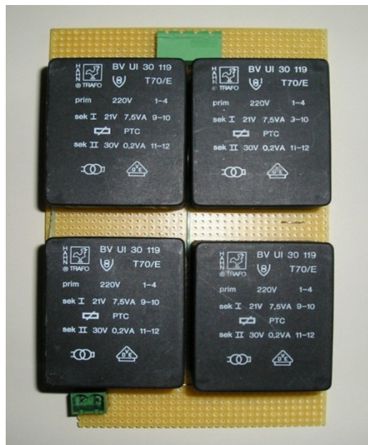
Figure 4.12 Transformer group for 230V voltage signal
