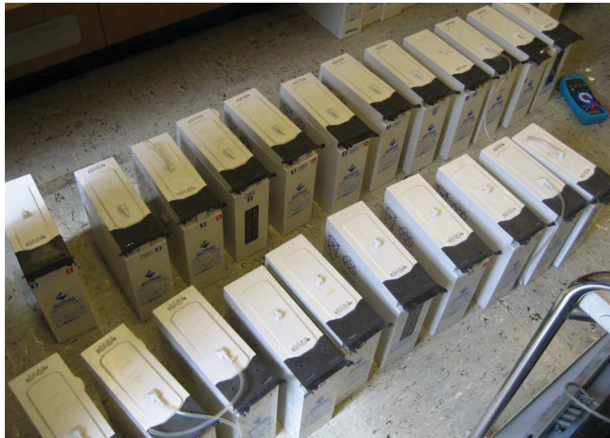
Figure 2.1: Pb Battery (Oerlikon) 12CP50 12V-50Ah
