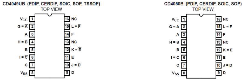
Figure 2.16: Connection diagram of CD4049 & CD4050
