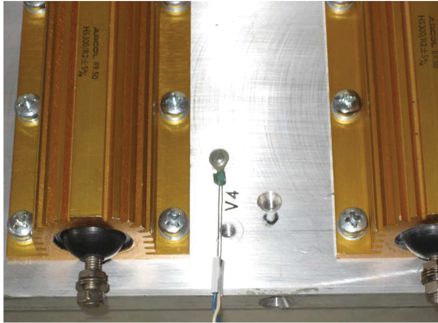
Figure 2.31: PTC and cooling device
