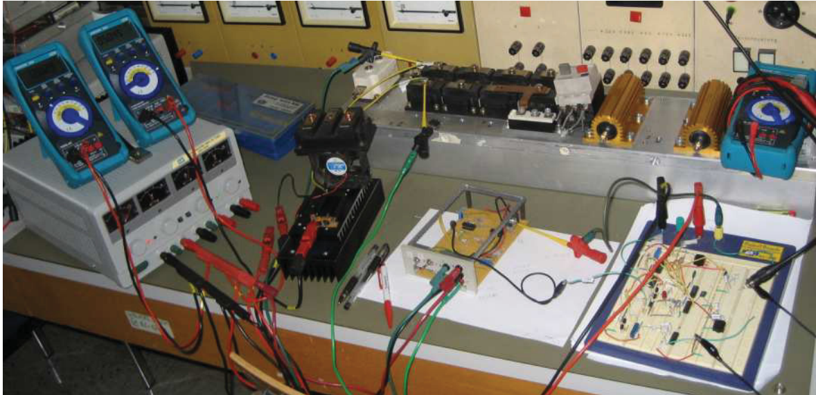
Figure 2.35: Battery discharge with timing system
