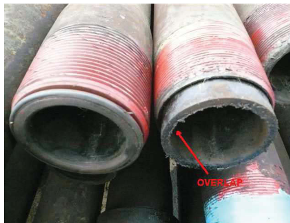
Figure 41 relined tubing after cutting the liner (right) and after creating a shoulder (left)
