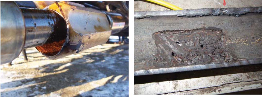
Figure 39 non-rotating centralizer and the impact on the tubing wall
