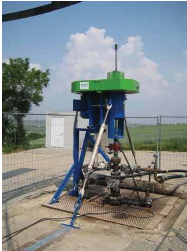
Figure 30 protection against vibrations for Drive Heads
