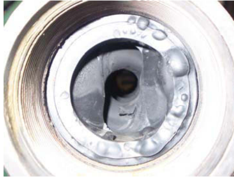
Figure 24 damaged stator elastomer, Pir 96a ,June 2008
