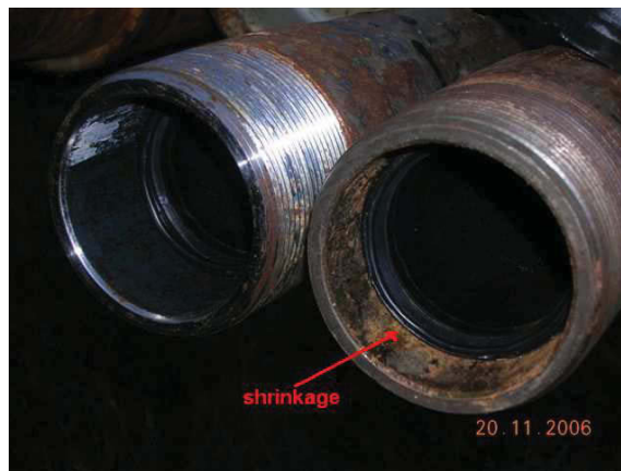
Figure 42 relined tubing with shrunk liner
