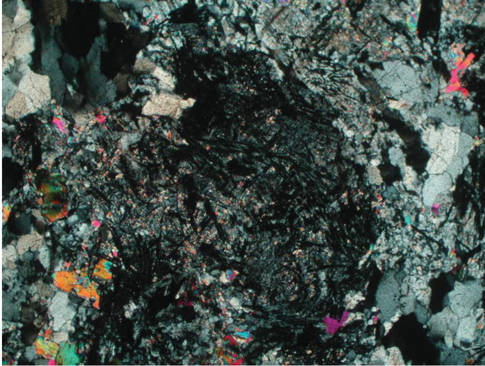
Figure 7-4: 'Needles' of clinozoisite in feldspar in the sample GG 1 CPLx4 (Picture size 75%).
