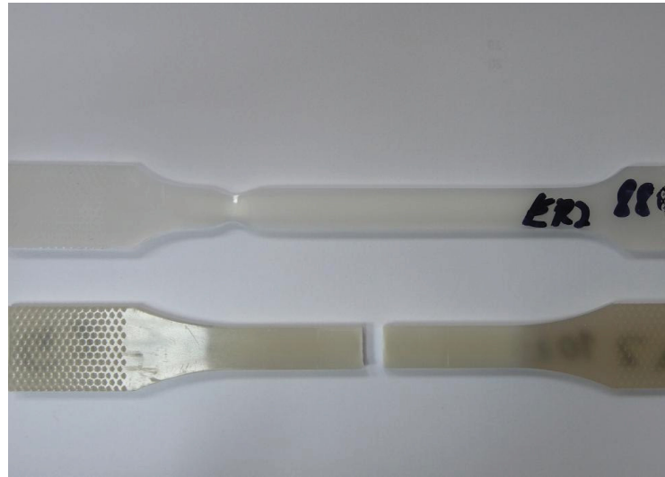
Figure 4.27: Ductile fracture with necking at ER2 (PP filled with 7 w% of polyolefin elastomer) at \sigma_{\max} = 24.5 MPa (top) and brittle fracture at material G2 (PP filled with 19 w% of glass spheres) at \sigma_{\max} = 26.75 MPa (bottom). Test conditions: R = 0.1 , 5 Hz, with ventilation, T_R \sim 20 °C.
