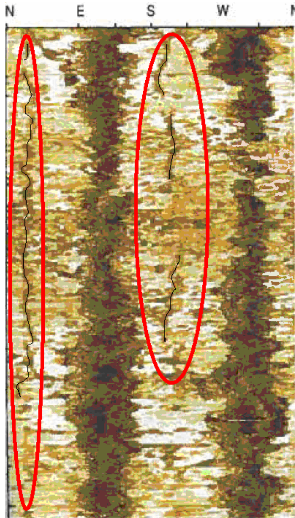
Figure 14, drilling induced tensile fractures 2
