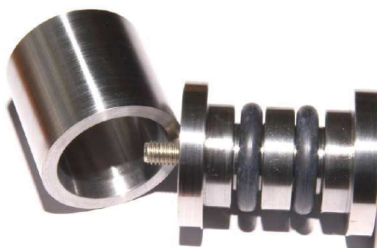
Figure 2.9: Constrained test set-up for two specimens
