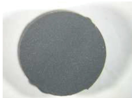
HNBR3 NORSOK: 0 no cracks
