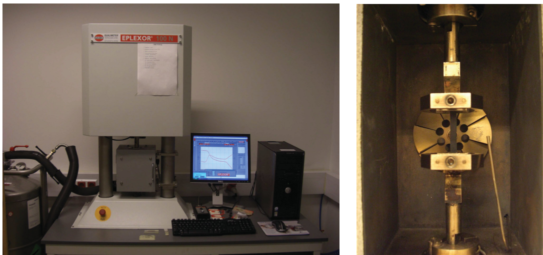
Figure 3.1: Test set-up for dynamic mechanical measurements
