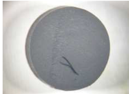
HNBR1 NORSOK: 1 single crack
