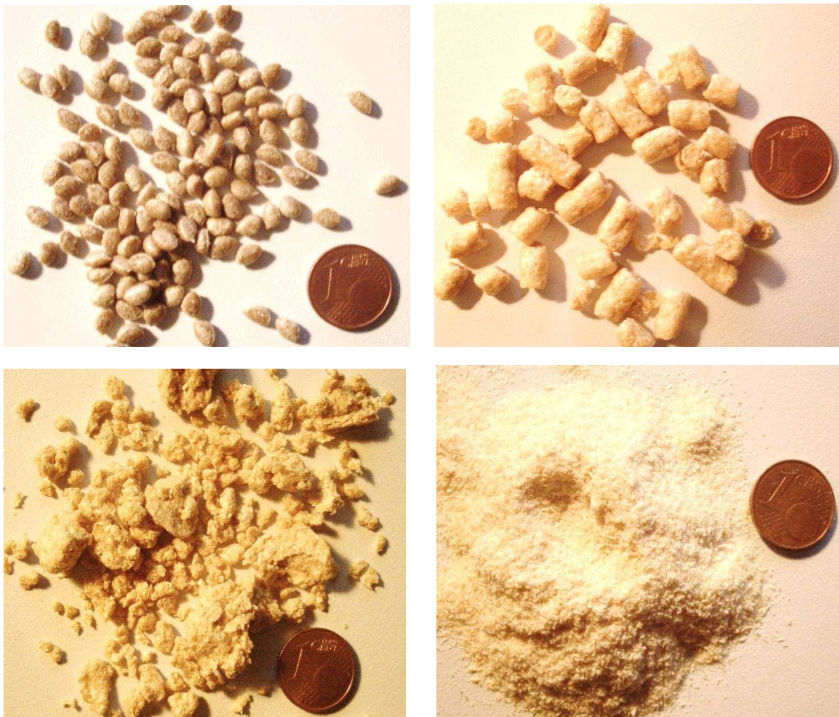
Figure 52: Optical comparison of all produced compounds. Compounder compound (top left), counter-rotating TSE compound (PP and PVC) (top right), PP agglomerate (bottom left) and PVC dryblend (bottom right).
