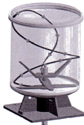
Figure 23: Mixer operating at high Froude number, trombe is fully developed (left), particle path in a fully developed trombe motion (right) [41, 44].
