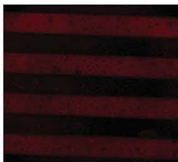
Figure 3.21: Optical micrograph of a thin film of PNOR-SCN after structured illumination ( 100\ \mu\text{m} grating) followed by post-treatment with \text{Ru}(\text{bpy})_2(\text{phen-5-NH}_2)(\text{PF}_6)_2 (CFM; \lambda_{\text{ex}} = 488\ \text{nm} ).
