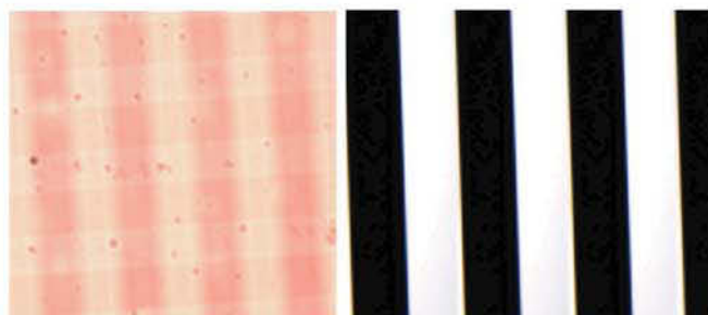
Figure 3.24: Dual-layer patterning of PVP- BZ and PVP- NA followed by \text{FeCl}_3/\text{NH}_4\text{SCN} post-modification (left); 100\ \mu\text{m} grating used as a contact mask for the photolithographic patterning (right).
