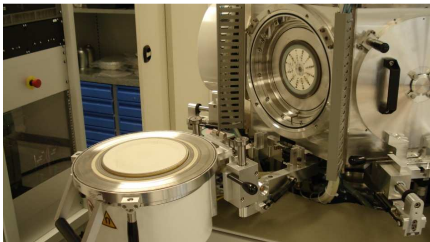
Figure 20: Sputtering Chamber of the Sprinter – 5 Coating System with a different target.
