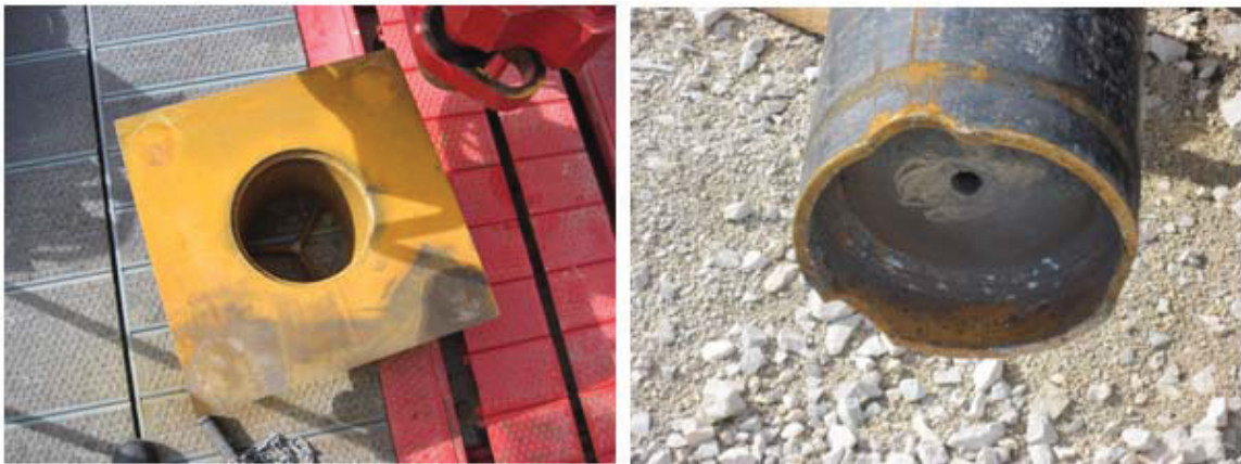
Figure 47: Insert plate (left) and casing modification (right) for the vibration test
