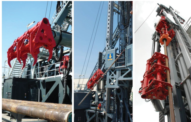
Figure 29 Working sequence of automated pipe handling system
