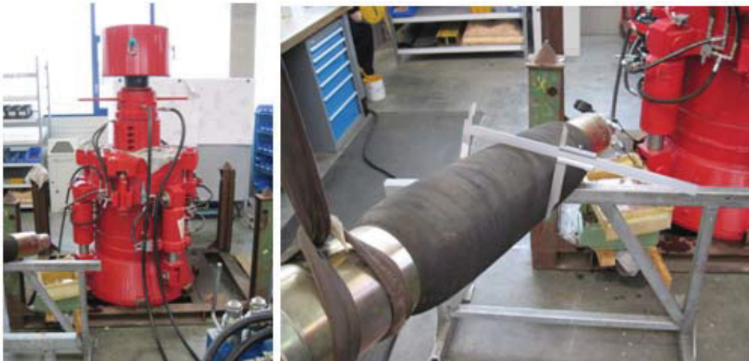
Figure 44: Test of the Casing Drive System and the Packer in the assembly shop
