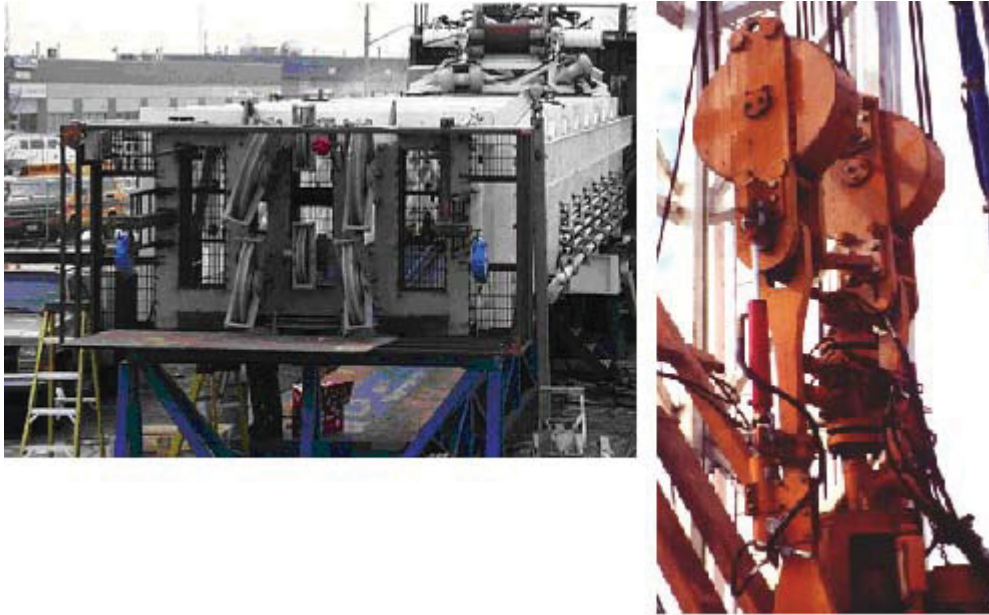
Figure 33: Split Crown Block (left) and Split Traveling Block with Wireline Blowout preventer (right) 60
