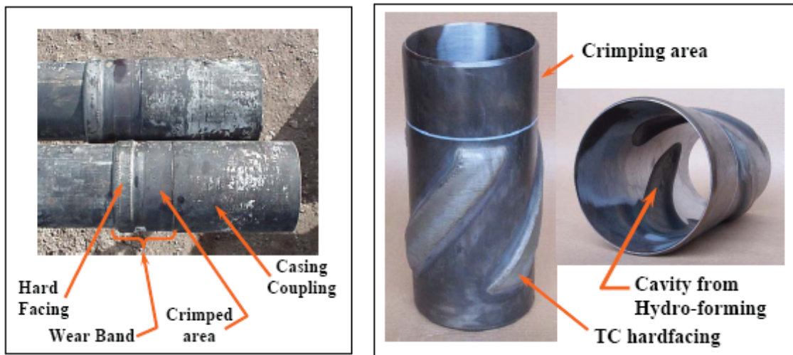
Figure 21: Casing wear protection methods 52
