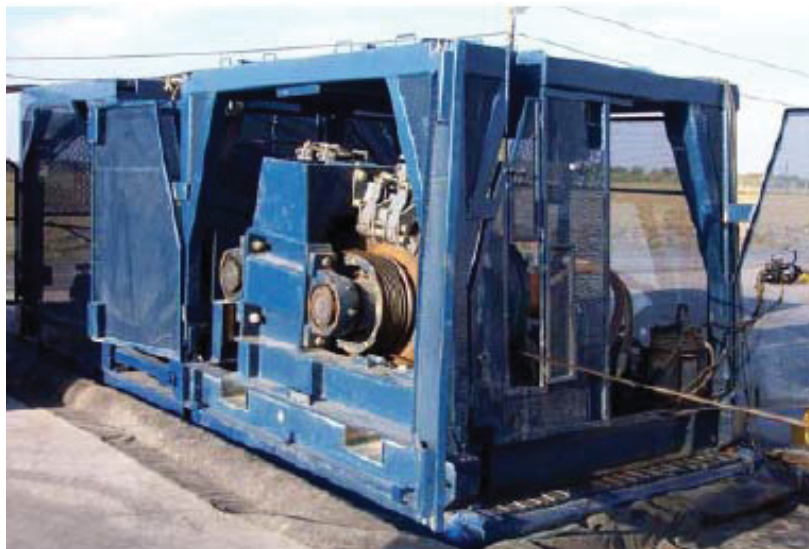
Figure 32: Special Casing Drilling Wireline Unit
