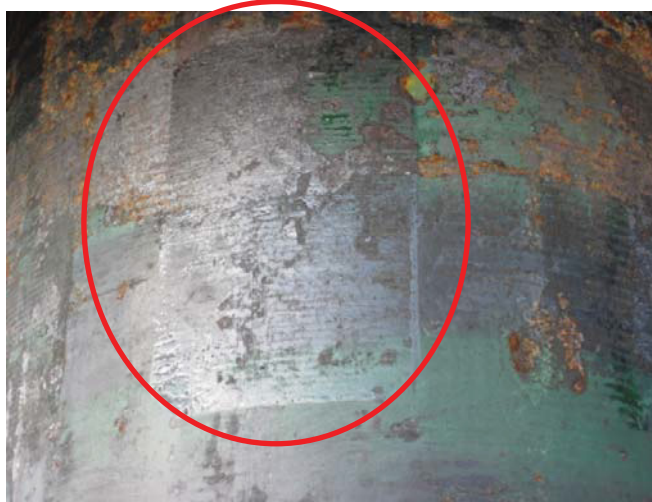
Figure 48: Mark of the clamping jaws with a closing pressure of 100bar
