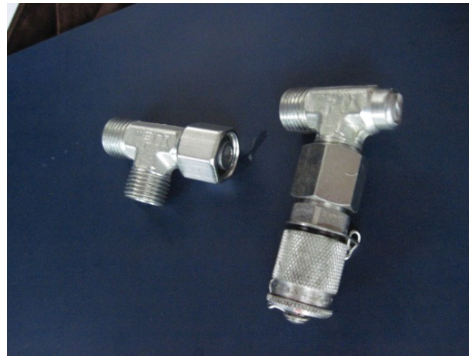
Figure 49: Hydraulic connection port (left: intact, right: broken)
