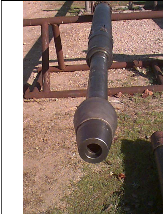
Figure 16: Rigid body (inflexible) expansion cone – Solid Expandable Tubular Applications, Brent Emmerson (Baker Hughes/2004) et. al.
