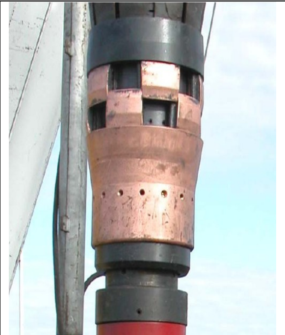
Figure 17: Inflatable (flexible) expansion cone – Expandable Monobore Drilling Liner Extension Technology, Carl Stockmeyer (Baker Hughes/2009) et. al.
