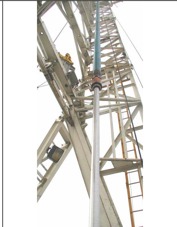
Figure 19: Hydraulic Stroker in extended position – Expandable System Overview, Carl Stockmeyer (Baker Hughes/2007) et. al.
