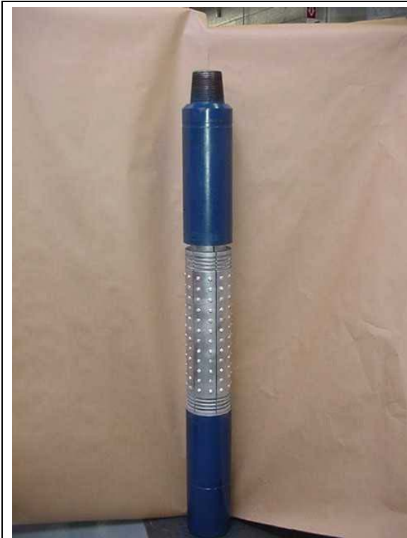
Figure 18: Hydraulic Anchor – Solid Expandable Tubular Applications, Brent Emmerson (Baker Hughes/2004) et. al.
