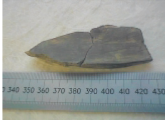
Figure 12: Angular caving shape from wellbore breakouts (W. Aldred et.al, 1999)
