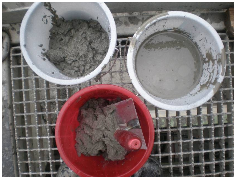
Figure 19: Increments from 12 ¼ in Hole Section: Cutting Sample (Upper Left), Mud Sample (Upper Right) and Sample of Flocculated Material (Bottom)
