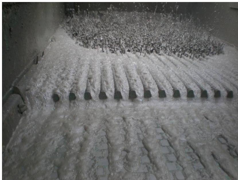
Figure 21: Very Fine Cuttings (from the 8 ½ in Reservoir Section) Flowing Over the Shale Shakers. Due to the Additive MIX II the Mud Appears to Be Foamy.
