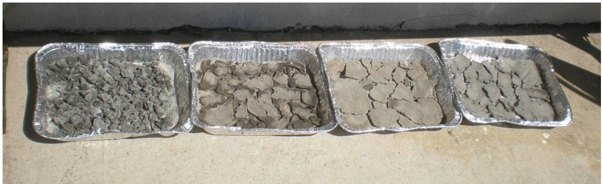
Figure 33: Picture from 2010/08/15 – Retain Samples from the Reservoir Section after Being Exposed to Natural Sunlight for ~ 2 Weeks (from Left to Right: Acidified Cuttings, Flocculated Material, Cuttings, Acidified Flocculated Material)
