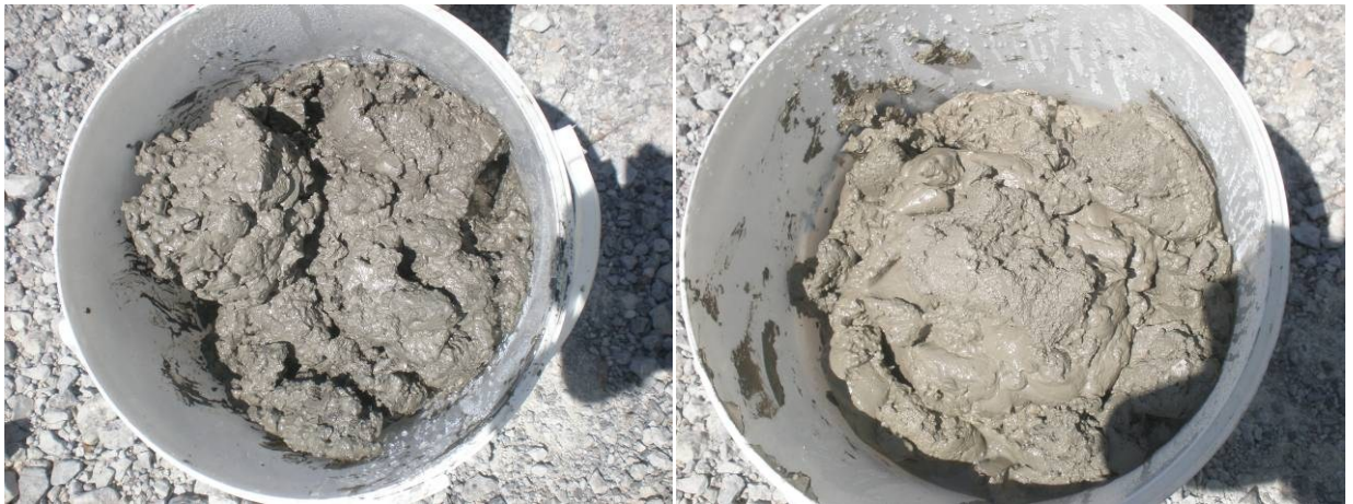
Figure 25: Cutting Sample (Left) and Flocculated Material (Right) from the Top Hole Section Where Bentonite Mud Was Used
