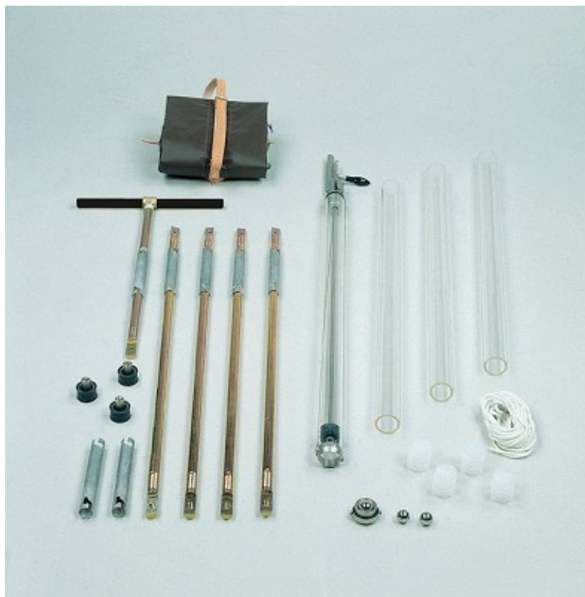
Figure 16: Sampling Device called ‘Multisampler’ (Saugbohrer) from the Company Eijkelkamp (32)
