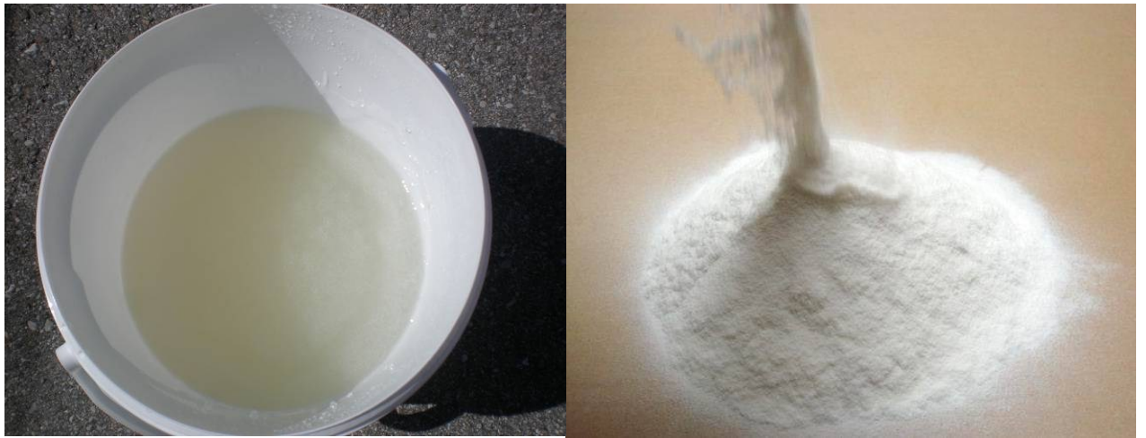
Figure 36: Freshly Mixed K 2 CO 3 -Polymer Mud (Left) and Powdered Polyanionic Cellulose Polymer Called Antisol (Right)
