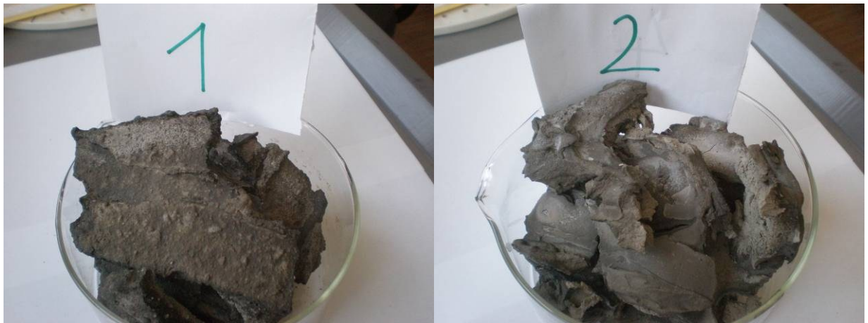
Figure 30: Dried Cuttings (Left) and Dried Flocculated Material (Right) from the Wiper tripping Run
