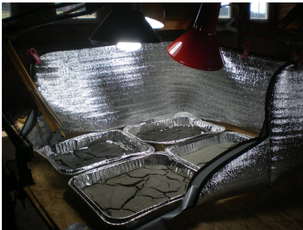
Figure 35: Picture from 2010/08/15 - Retain Samples from the Reservoir Section After Being Exposed to Artificial Sunlight for ~ 2 Weeks: Flocculated Material at Front Left, Cuttings at Front Right, Acidified Flocculated Material at Rear Left, Acidified Cuttings at Rear Right
