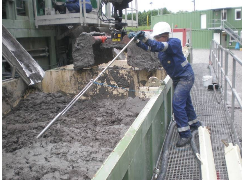
Figure 22: Sampling of Flocculated Material from the 8 ½ in Reservoir Section. The Samples Were Taken Out of the Container with the Help of the Multisampler from Eijkelkamp.
