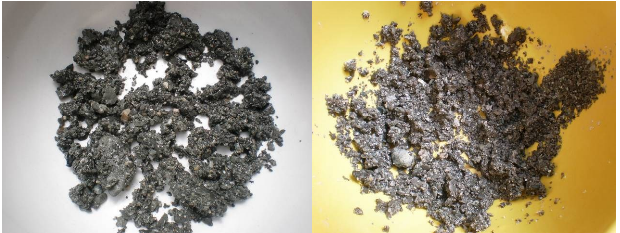
Figure 27: Washed and Sieved Cutting Samples from the Wiper tripping Run (Left Picture) and from the Reservoir Section (Right Picture)
