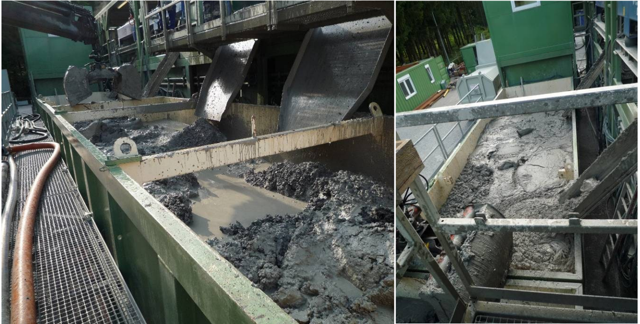
Figure 13: Pictures of the Cutting Boxes (Left Picture - Outlets of Shale Shakers, Right Picture – Outlets of Centrifuges)
