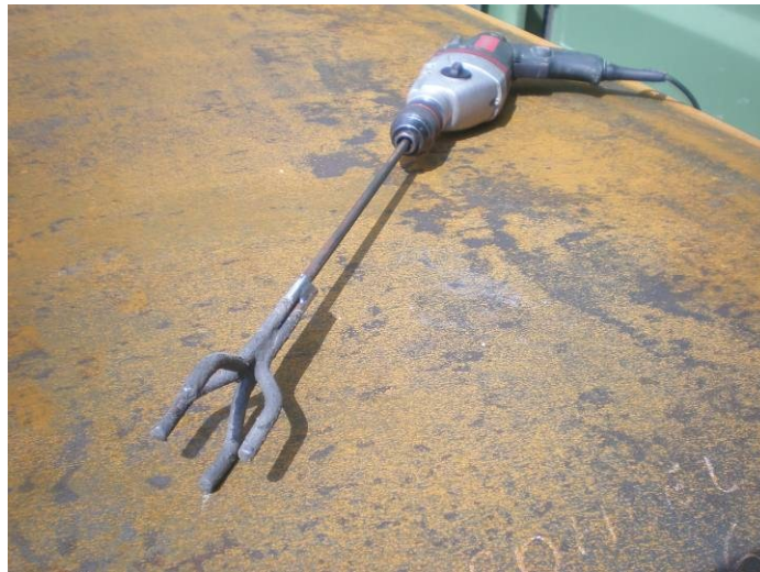
Figure 26: Self-Made Blender Wand Attached to an Electric Drill
