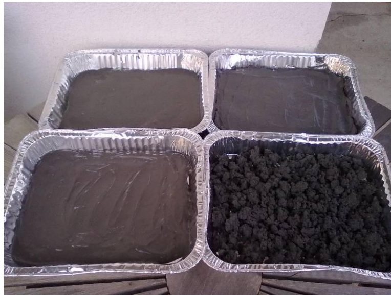
Figure 32: Picture from 2010/08/03 – Retain Samples from the Reservoir Section When Exposition to Natural Sunlight Started (Flocculated Material at Front Left, Acidified Cuttings at Front Right, Cuttings at Rear Left, Acidified Flocculated Material at Rear Right)
