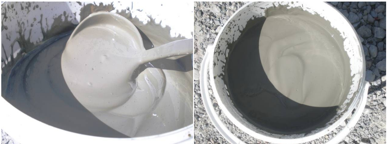
Figure 24: Bentonite Mud Sample – Note the Viscous and Thixotropic Nature of the Mud
