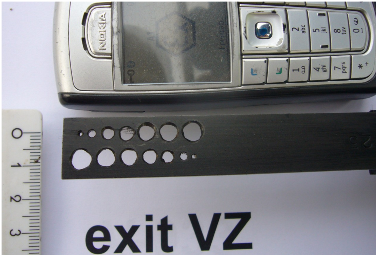
Picture 16: Scale coupon of VZ exit 15 days after installation (wiped clean with woven felt)
