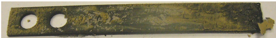
Picture 11: Dried coupon from the sealed jar with SI-4041
