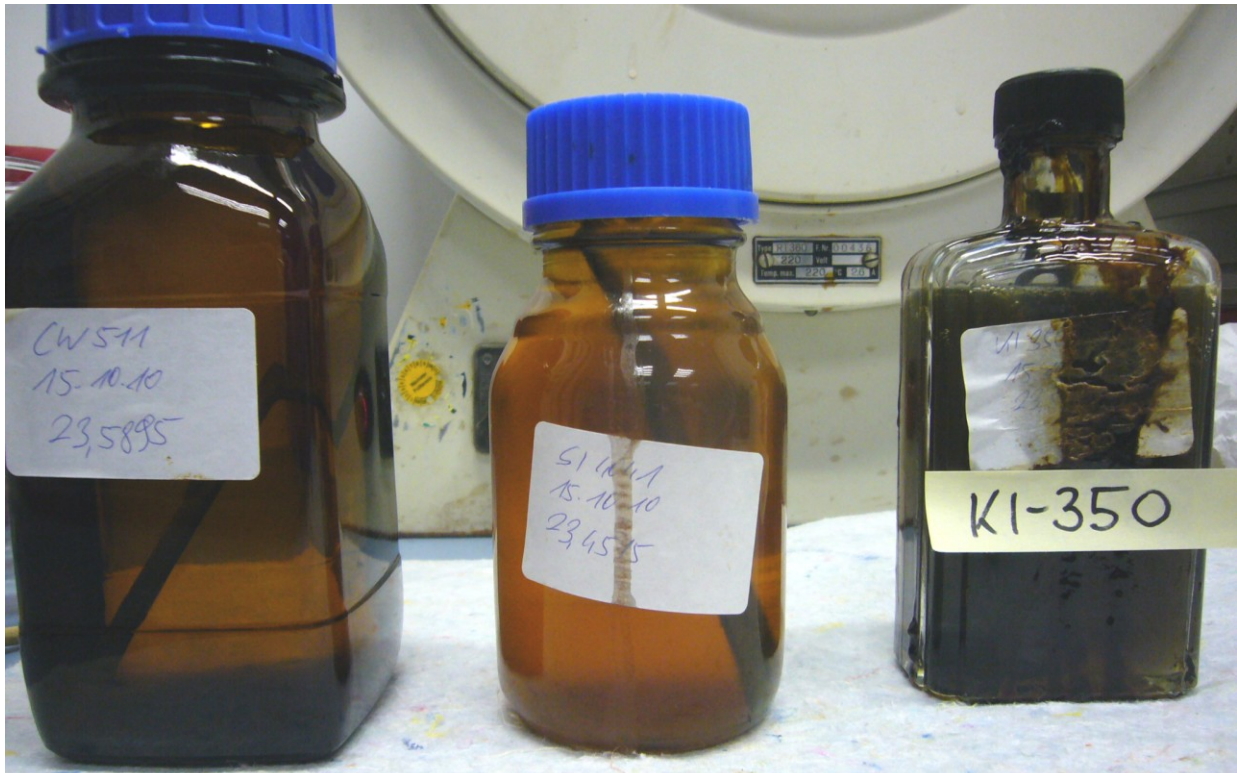
Picture 8: Sealed glasses with corrosion coupons in pure CW511, SI-4041 and KI-350
