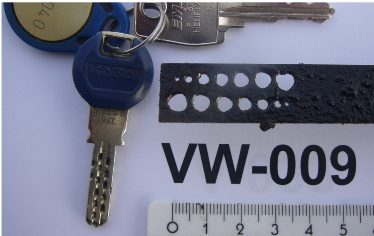
Picture 15: Scale coupon of pre-pressurization module VW-009 15 days after installation
