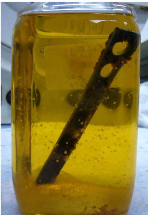
Picture 4: Open glass with corrosion coupon in CW511
