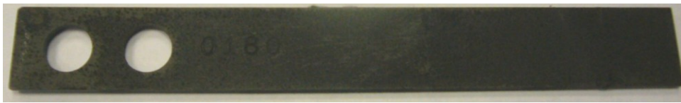
Picture 10: Dried coupon from the sealed jar with CW511
