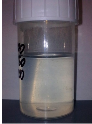
Picture 21: Precipitations (KI-350: 200ppmv, CW511: 150ppmv, SI-4041: 200ppmv)
