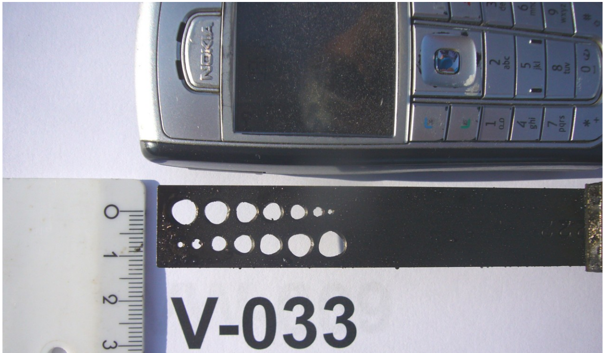
Picture 14: Scale coupon of producer V-033 15 days after installation
