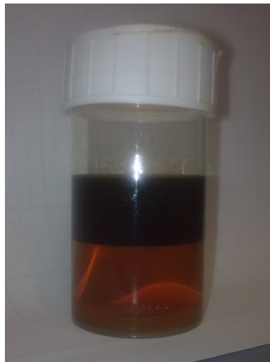
Picture 22: Mixture of concentrated inhibitor liquids (KI-350, CW511 and SI-4041)
