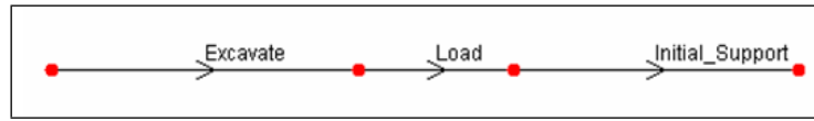
Figure 5.20: Activity Network Modeling the "Excavation" Subpart of the "Construction Model" for Conventional Tunneling
