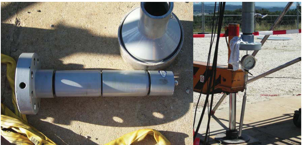
Figure A 12-5 LEFT: Capillary Hanger; RIGHT: Cap.-Hanger, Pressure Gauge and Injection Valve
