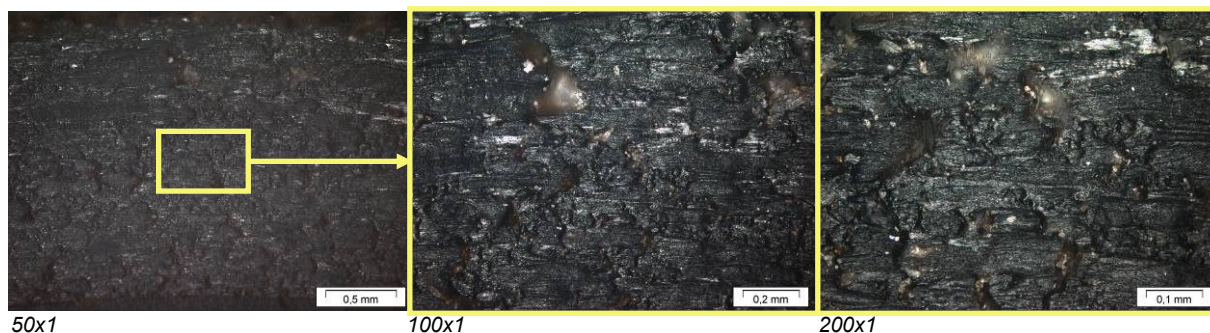
Figure 4.3-2: Micrographs of unfilled specimen's wear track (Constant load test, p=1 MPa, v=100 rpm, t=4 h, Test No. 1)
