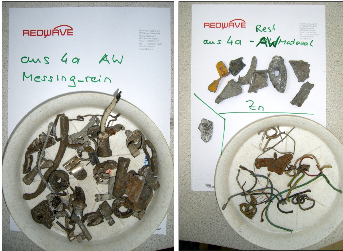
Figure 52 Photographs of Test 4a- Ejection, brass_pure (left), Zn-pieces (right-top), wire (right-bowl), Cu/Zn-piece (right-left)
