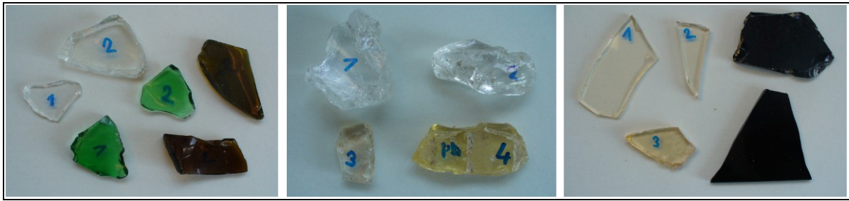
Figure 43 Samples, “normal culets”(left), leaded glass (middle), heat resistant glass (right)
