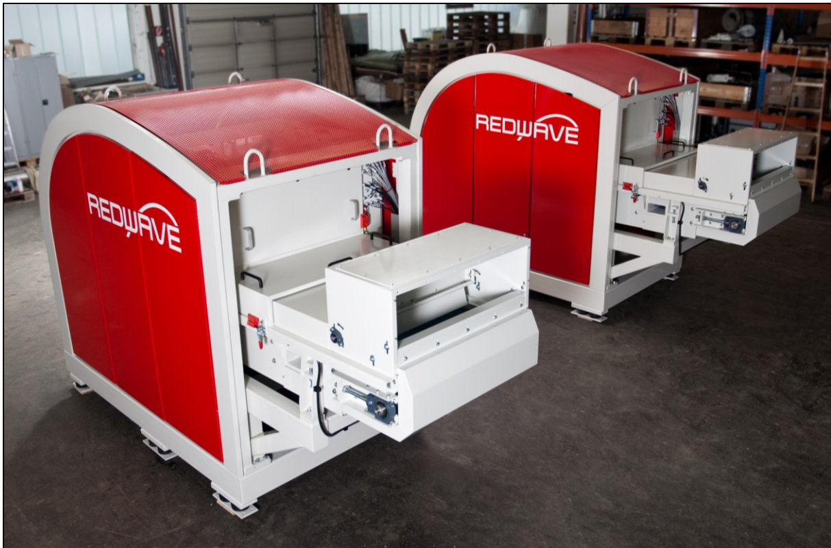
Figure 24 Commercial used REDWAVE XRF-system (without vibratory feeder)
