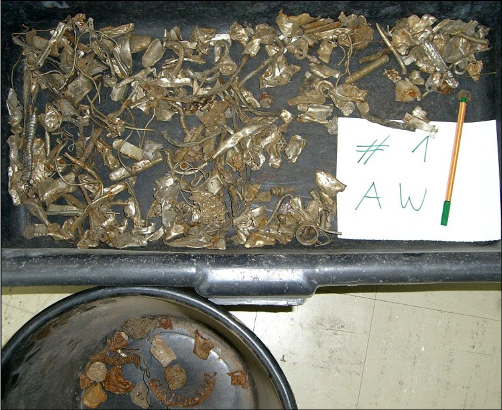
Figure 46 Photographs of Test 1- Ejection, CRES (top), Impurity (bottom)
