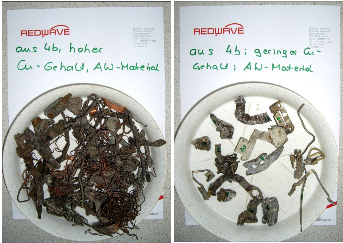
Figure 54 Photographs of Test 4b- Ejection, Cu_pure (left), Cu-pieces (right)
