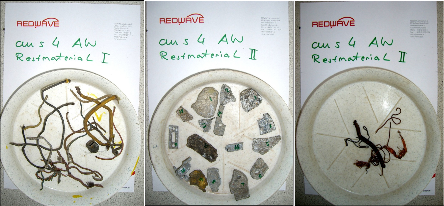
Figure 51 Photographs of Test 4- Ejection, wire (left), miscellaneous pieces (middle), Cu-pieces (right)
