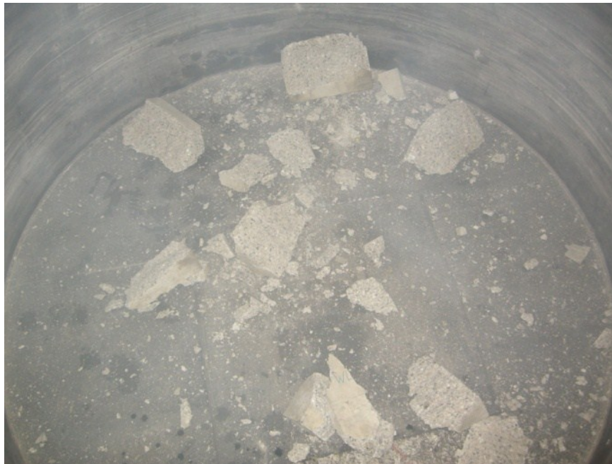
Figure 27: WLM-40-03 test block; after blasting
