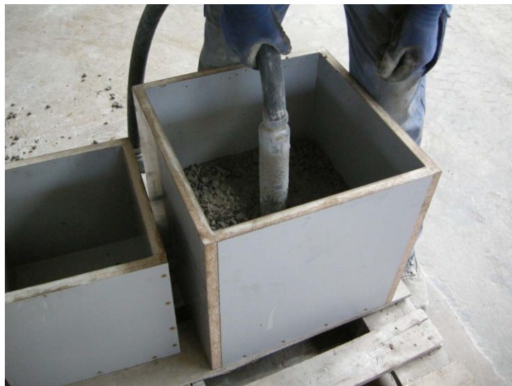
Figure 21: Formworks while filled and compacted
