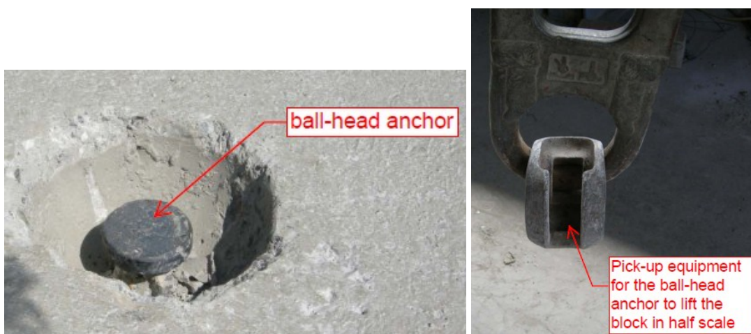
Figure 23: Ball-head anchor and lift system
