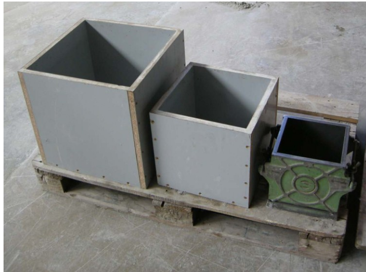
Figure 20: Formworks for the samples in laboratory scale
