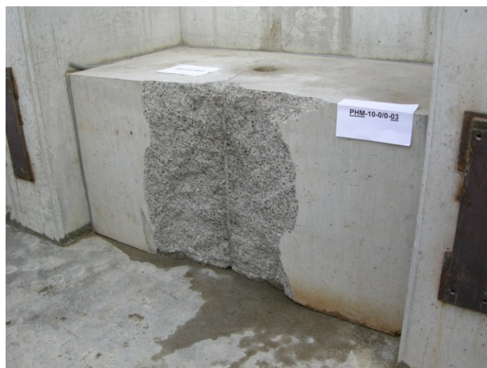
Figure 30: PHM-10-03 test block; after blasting
