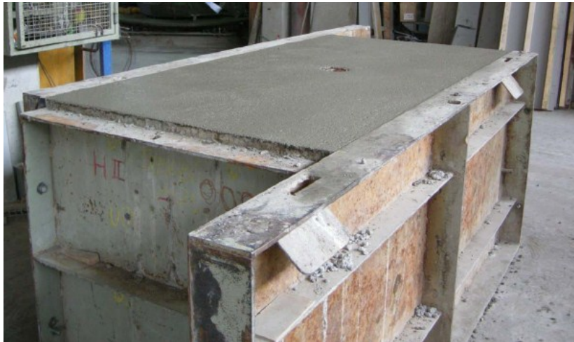
Figure 22: Formworks for the samples in half scale
