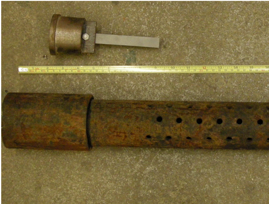
Background Data 18 – Example Picture of Downhole Coupons Installation in Tailpipe
