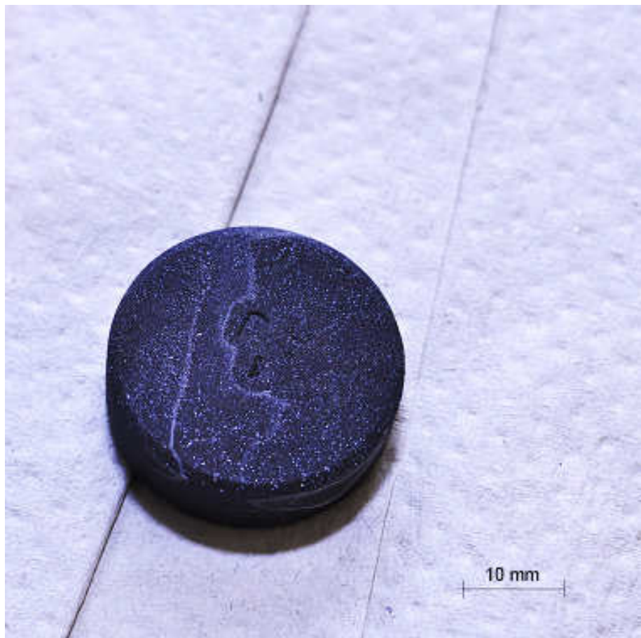
Background Data 34 – FeCO 3 layered Sample representative for all Samples after Exposure to 120 °C Environment
