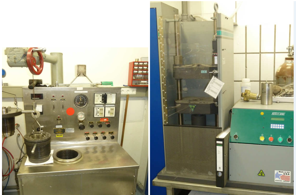
Figure 7.7 - Pressure/temperature cell (left) and compressive strength tester (right)
