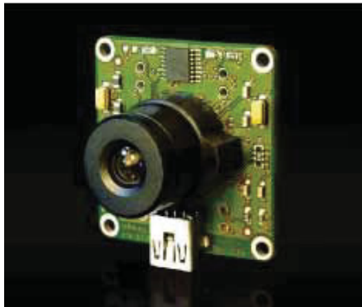
Figure 2.11: The VRmagic VRmC-9+ COB (b/w) is a 1/2" grayscale industry approved camera with a resolution of 1280 \times 1024 pixel. The resolution must be high enough to catch all the details, as the whole target object is pictured at once. Tested objectives are a normal-angle lens with f = 12mm and a wide-angle lens with f = 3.6mm .
