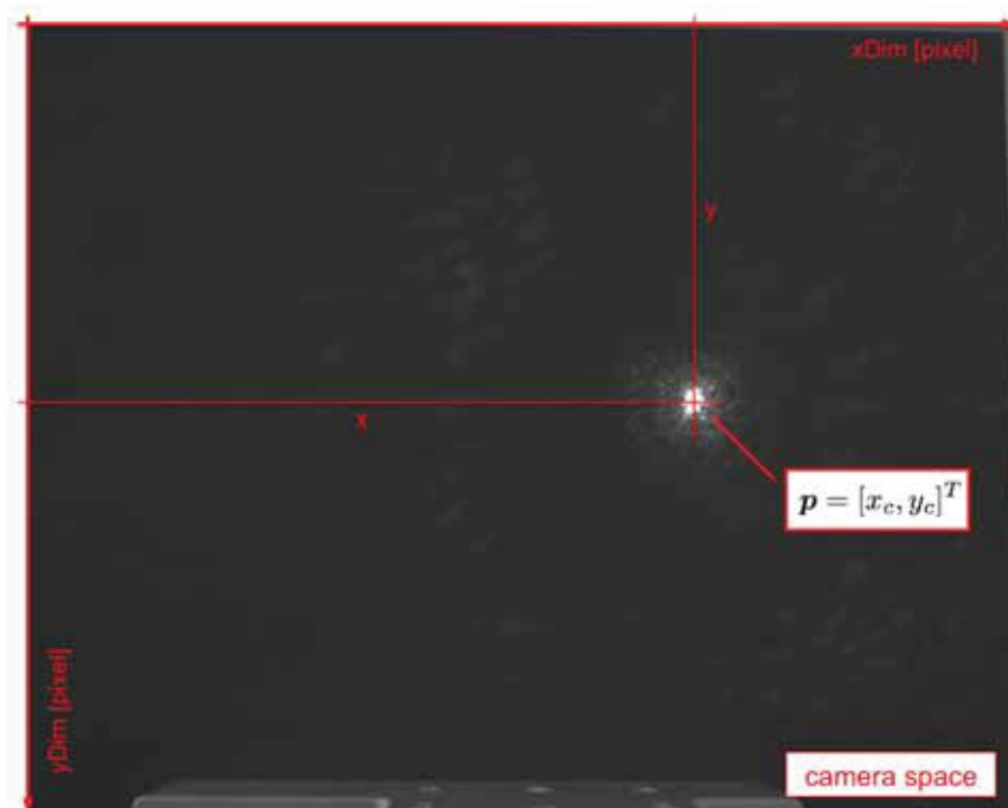
Figure 1.4: The camera space is biased because of optical effects. A mathematical relation is established through coordinate mapping methods, which are able to transform the coordinates of \mathbf{p} to its real world pendant \mathbf{q} . Distances are measured in pixels.
