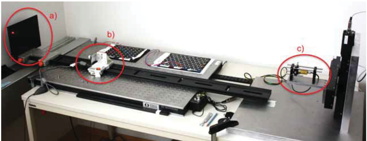
Figure 2.10: The prototype consists of a target plate a), a camera b) and a laser c). A measurement station is composed of a) and b), whereby both parts are unchangeably attached to a carrier cantilever to keep the relative distance static. The laser c) is mounted on a xy-table (there's also a setup with a linear drive) to enable relative movements between the laser beam and the measurement station.
