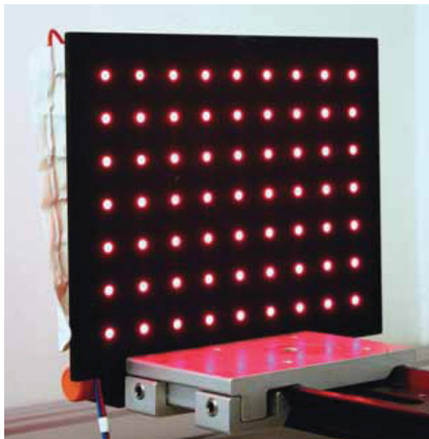
(a) The calibration plate features 63 LEDs.
