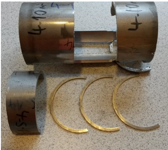
Fig. 6: Sample cup with cut-out half rings
