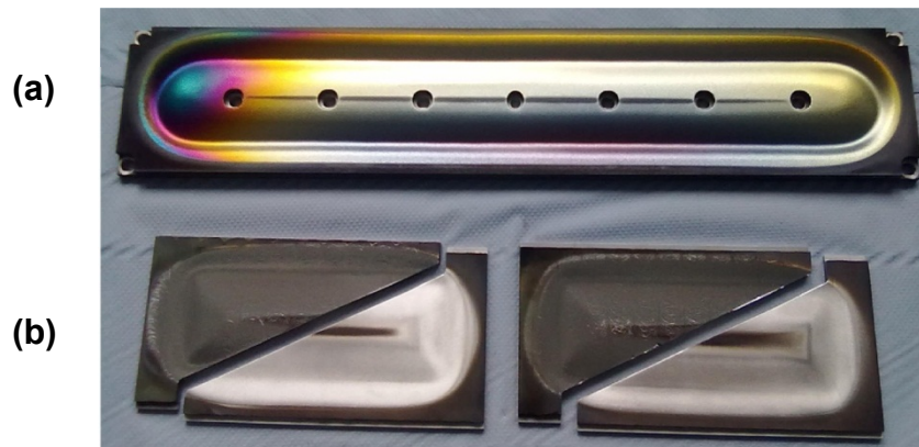
Fig. 4.1: (a) Standard sized TiAl compound target and (b) segmented Cr and Al target, respectively.
